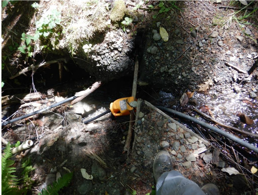
Photo 23—Stream diversion fabricated using a juice bottle at WQ 11.
