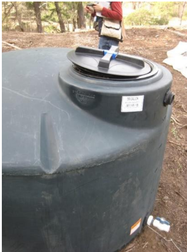
Chemical mix tank with top partially covering tank and drain valve open. Photo 26 provides a view inside of the tank.
