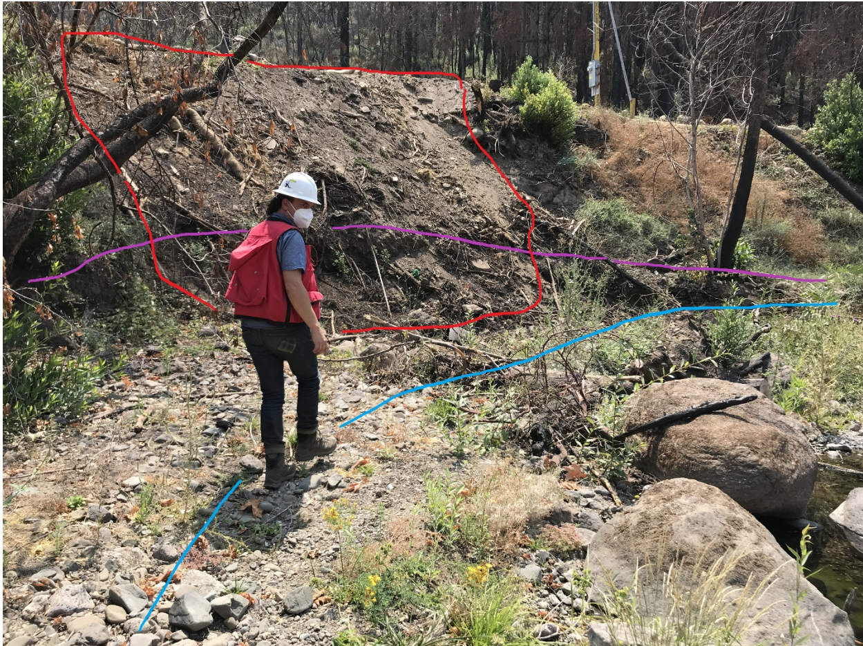
Figure 2. View of discharge from within channel of unnamed tributary. Red line: approximate extent of discharge. Purple line: approximate bankfull. Blue line: Approximate path of side channel during higher flows.
