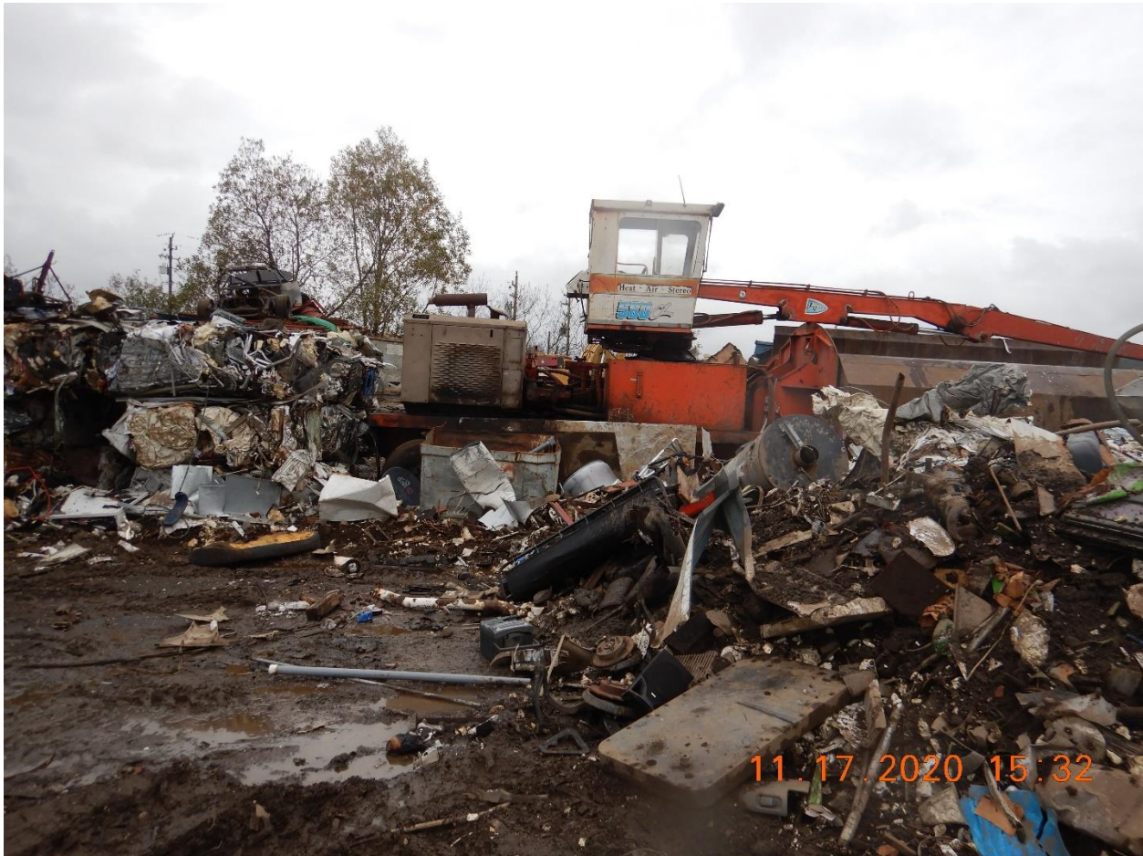
Picture 5 – View of debris, trash and scrap metals stored outside directly on the ground with no cover. Source control and housekeeping practices are not implemented throughout the facility. Picture taken by Farzad Kasmaei.
