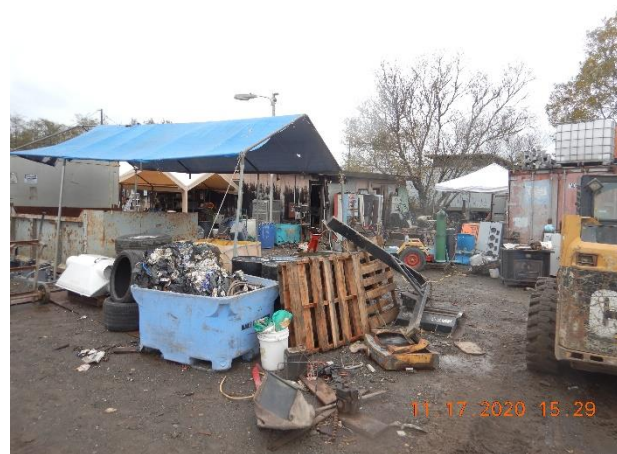
Pictures 3a, 3b – View of metal parts that are stored outside in the bins with no covers (lids) and exposed to rain. Source control is not implemented. Pictures taken by Farzad Kasmaei.
