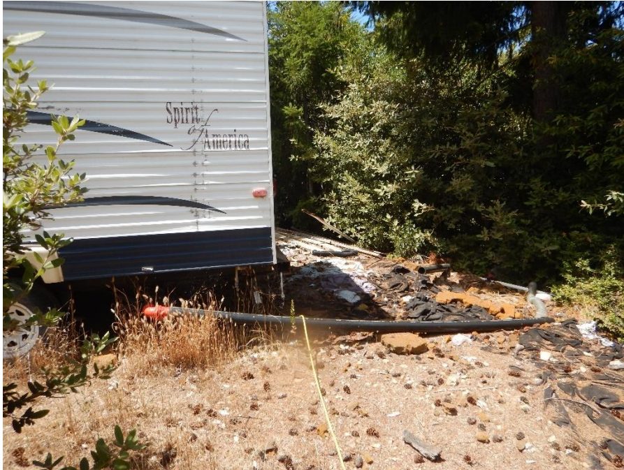
Photo 3: LL2: RV with outlet pipe discharging to ground
