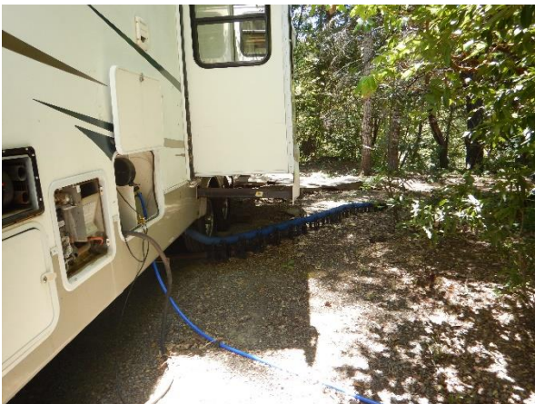
Photo 5: View of greywater pipe from an RV located near the residence.
