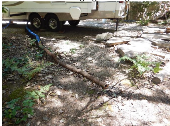
Photo 6: Closer view of greywater pipe from an RV discharging to the ground.
