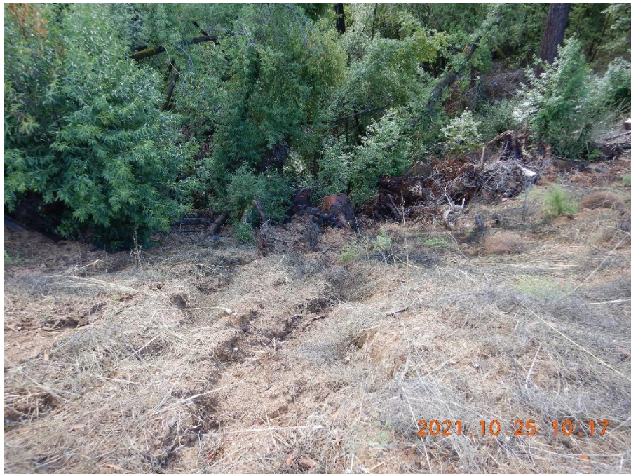
Photo 8—Looking east and downslope from WQ5. Staff measured a length of 47 feet with a tape measure from the edge of the graded pad to the slash at the bottom of the rills in the middle of the image and measured a horizontal distance of 39 feet between the two points with a gps device resulting in a local slope of 67 percent.
