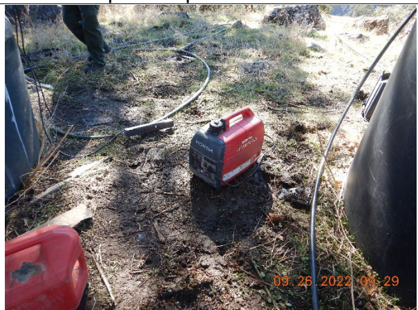
Photo 22 – uncontained generator and gasoline tank at WQ4
