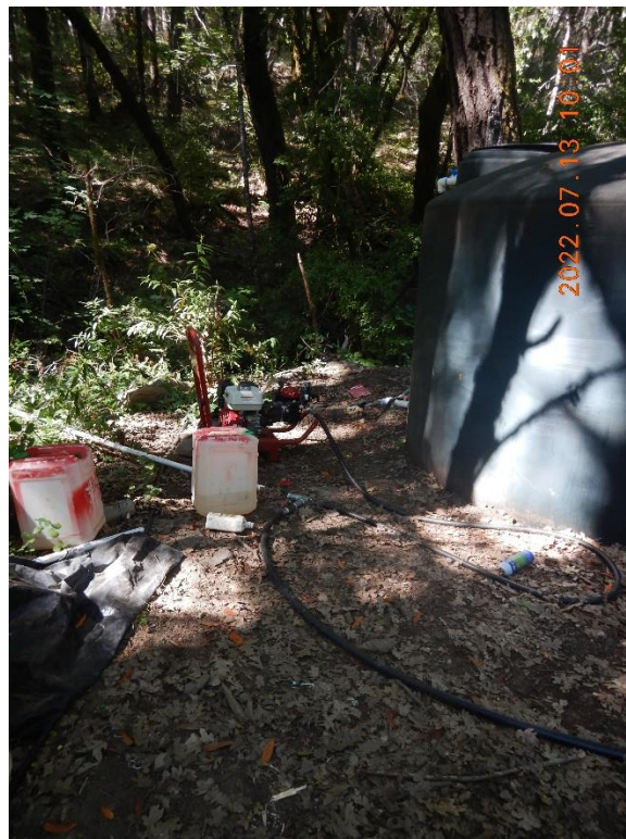
Figure 62. WQ13, WP 782. A streamside landing is being used to facilitate water diversion for the cultivation. Two pumps and a water tank are located on the top of the bank of Cold Creek. There is a diversion into the tank, and out are two pumps, each on separate out lines.
