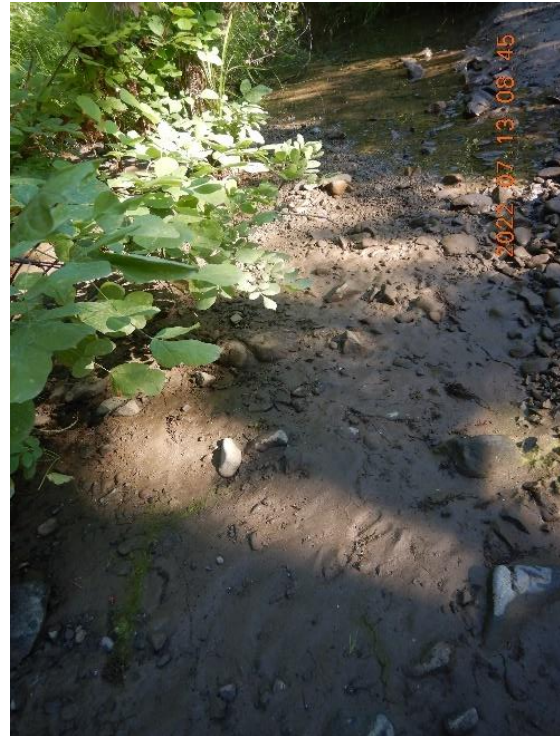
Figure 14. WQ2, WP769, X1. Fine sediment deposited in watercourse immediately downstream of ford crossing from road-related erosion of the crossing and the hydrologically connected road approaches.
