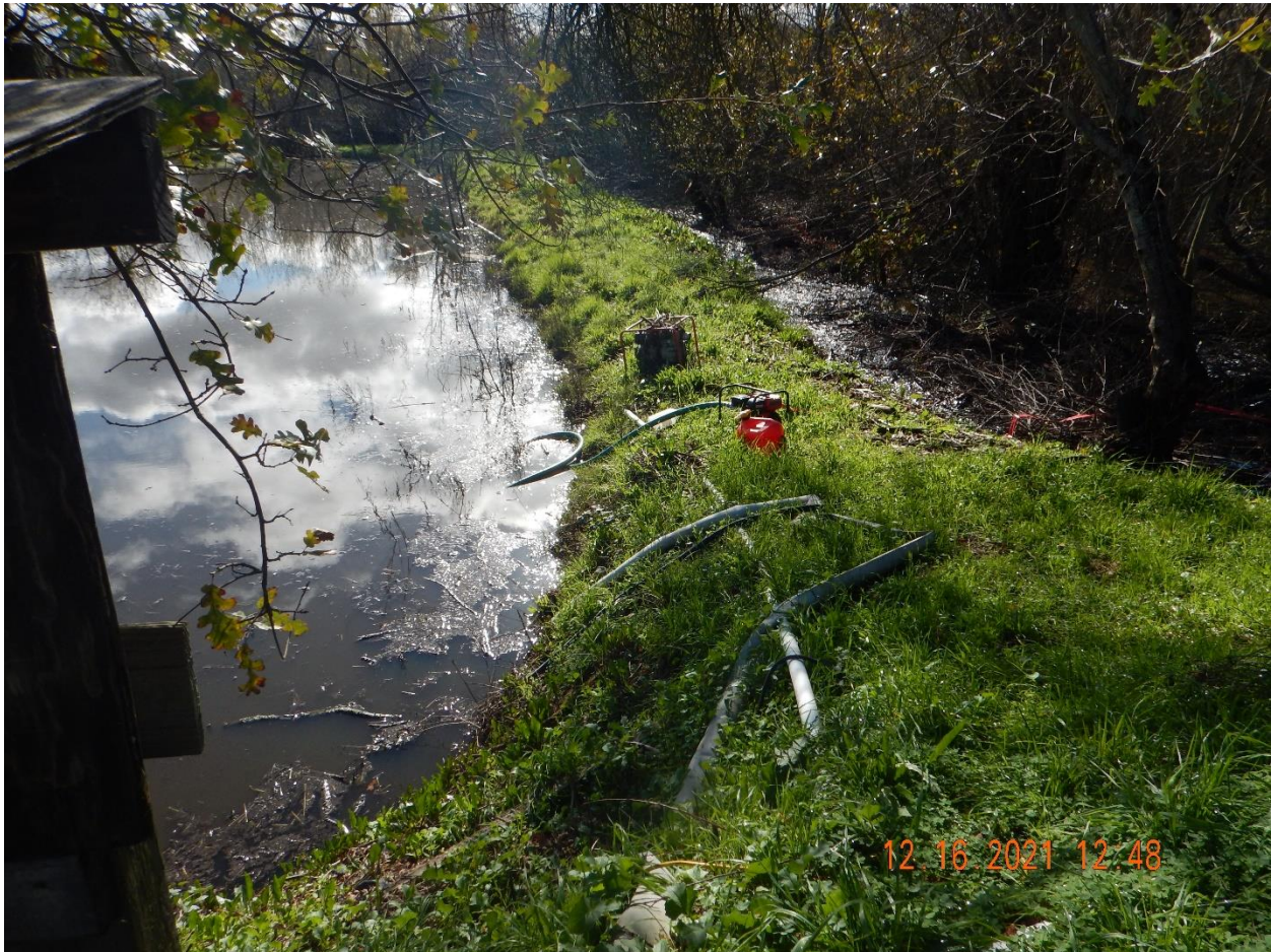
Photo 13- West berm of south irrigation field, with portable pumps, gas can, and orange discharge hose to Atascadero Creek. Photo taken facing south from berm between Pond 3 and south irrigation field.
