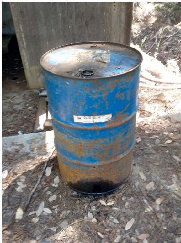
Photo 16—Looking east at a leaking 55-gallon drum outside of the generator shed at WQ10. The drum is on top of a piece of plywood and surrounded by leaf litter. Oil is visible on the ground at the bottom of the drum.
