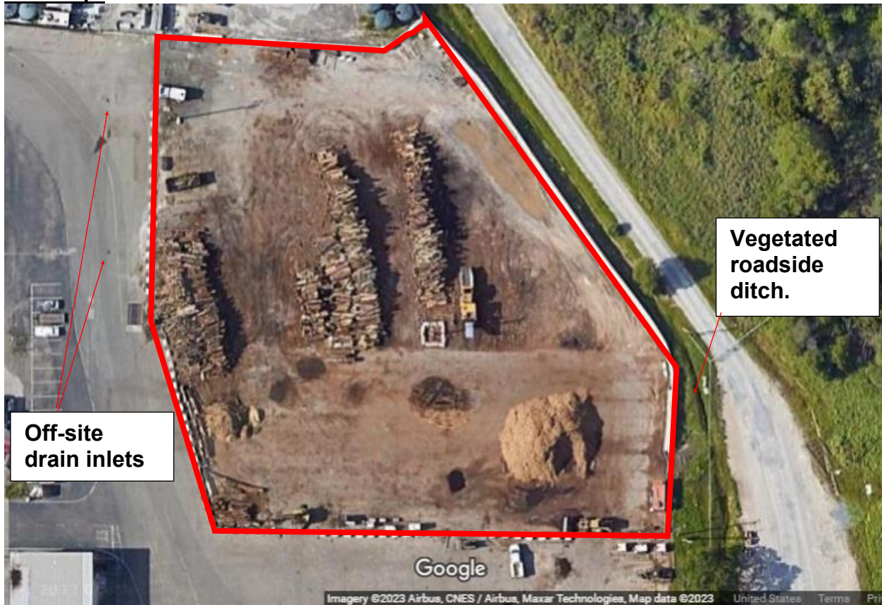
Picture 10 – Site map indicating the Facility’s boundary and existing roadside ditch and off-site drain inlets.
