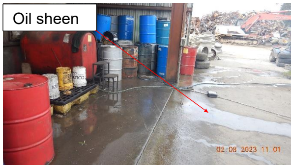
Pictures 17a, 17b – View of the fueling storage area. Oil sheen was observed within this area. No BMPs were present. Picture taken by Farzad Kasmaei.
