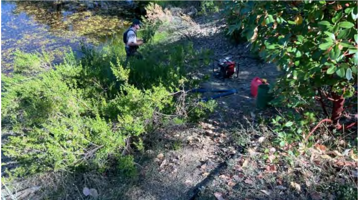
Figure 5. Gas pump located on the berm of the pond at Polygon Location 1; I did not observe measures to ensure petroleum is prevented from discharge to land and to the pond.
