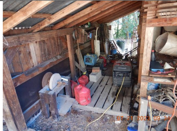
Photo 14 – partially properly stored petroleum products near WQ9. Some gasoline containers and others are on bare ground
