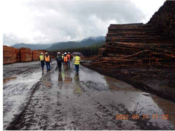
Pictures 3c and 3d: Large material stockpiles located within the log deck area of drainage area 1 exposed to rain. This paved area is covered with many inches debris, mud, wood fiber. No BMPs are present. Picture taken by Heaven Moore.
