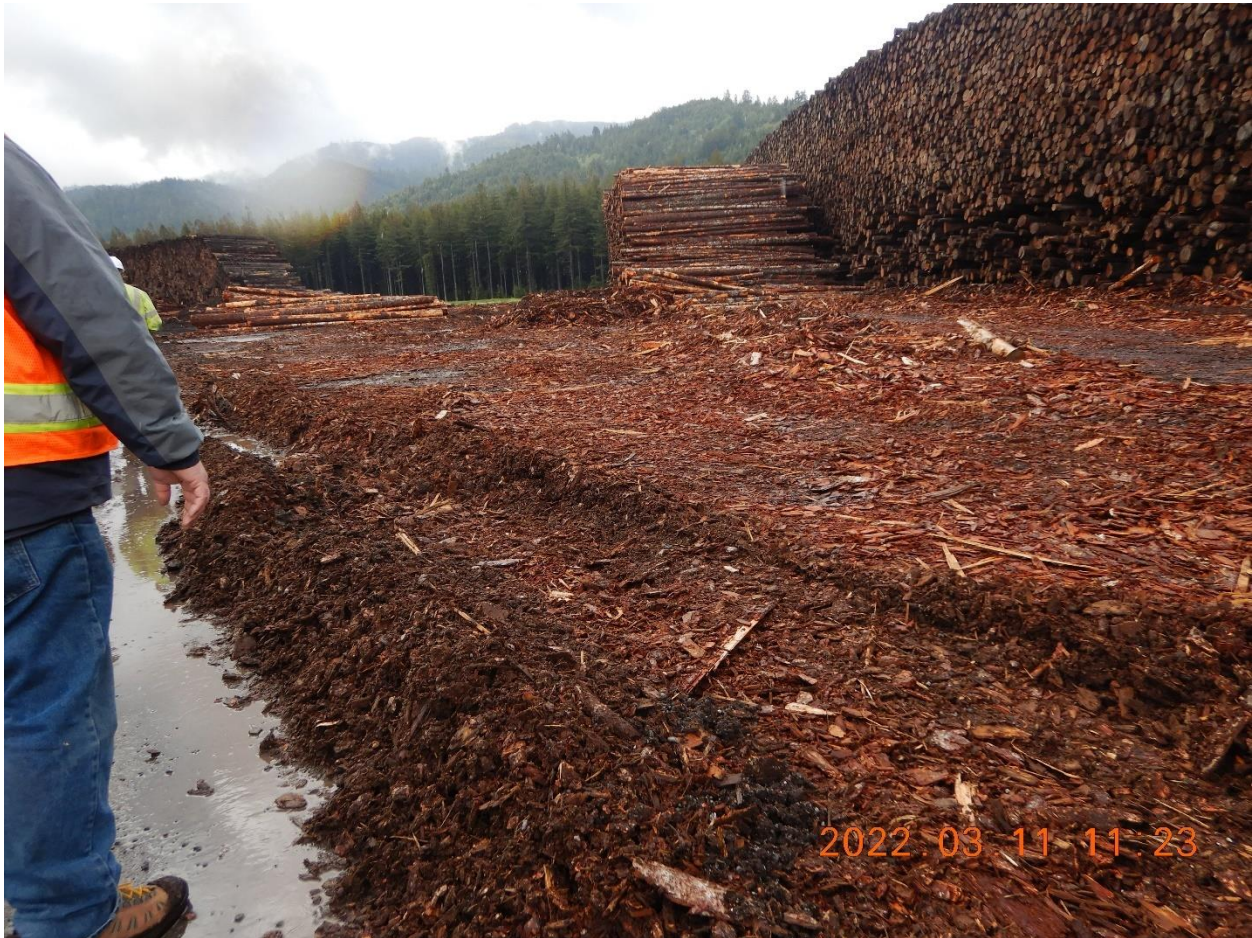
Picture 3e: Large material stockpiles located within the log deck area of drainage area 1 exposed to rain. This paved area is covered with many inches to feet of debris, mud, and wood fiber. No BMPs are present. Picture taken by Heaven Moore.
