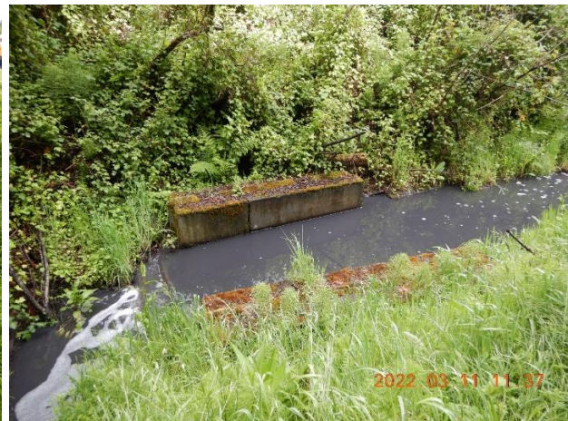
Pictures 6g and 6h: Picture discharge from the retention pond to the Eel River. The discharge appeared to be highly turbid, dark, and had a gray hue. Foam was observed on the surface. Pictures taken by Heaven Moore.
