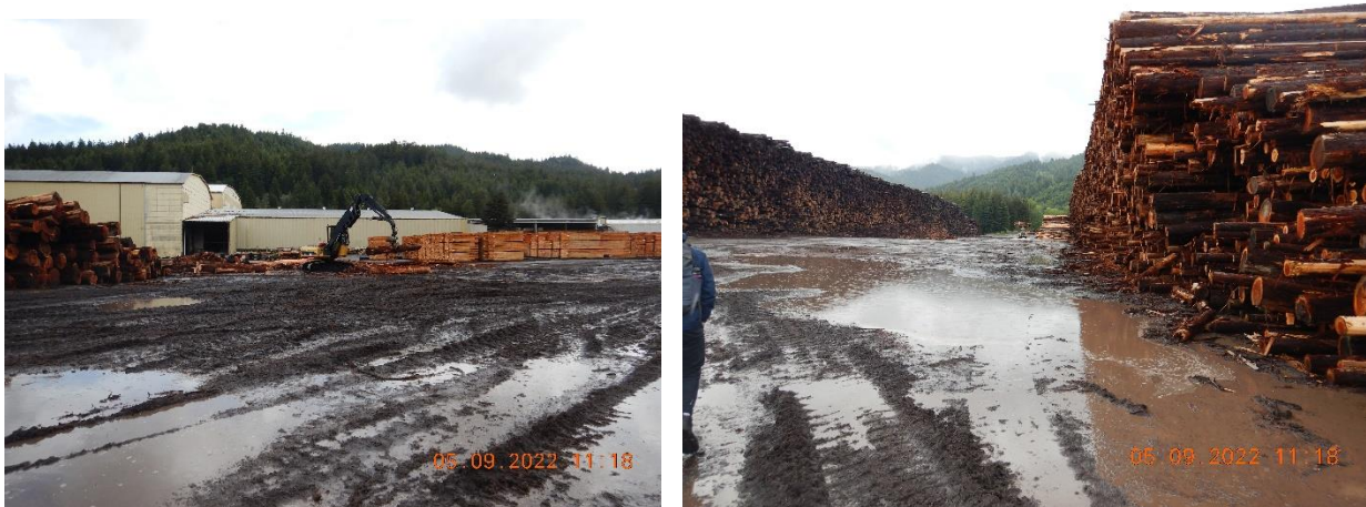
Photo 4a and 4b: View of highly turbid runoff and thick mud on the paved log deck. Picture taken by Farzad Kasmaei.
