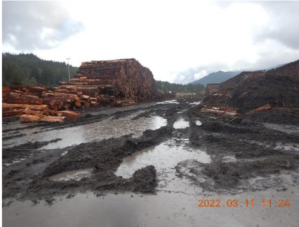
Pictures 2h and 2i: Large industrial waste material piles and stockpiles located within the log deck area of drainage area 1 exposed to rain. This paved area is covered with many inches debris, mud, wood fiber. No BMPs are present. Picture taken by Heaven Moore.
