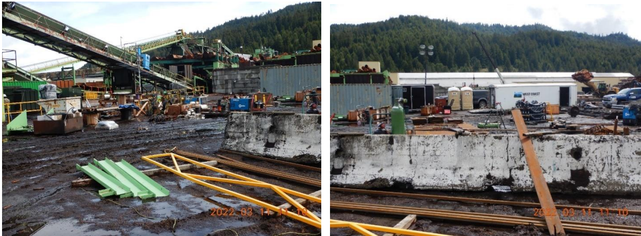
Pictures 2a and 2b: Industrial equipment, materials, and waste located within drainage area 1 exposed to rain. This paved area is covered with many inches debris, mud, wood fiber. No housekeeping BMPs or inlet protection BMPs are present. Picture taken by Heaven Moore.
