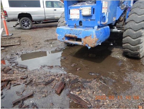
Pictures 2d and 2e: Industrial equipment and associated oil sheen in drainage area 1 exposed to rain. This area is covered with many inches debris, mud, wood fiber and directly adjacent to unprotected storm drain inlets. No housekeeping BMPs or inlet protection BMPs are present. Picture taken by Heaven Moore.
