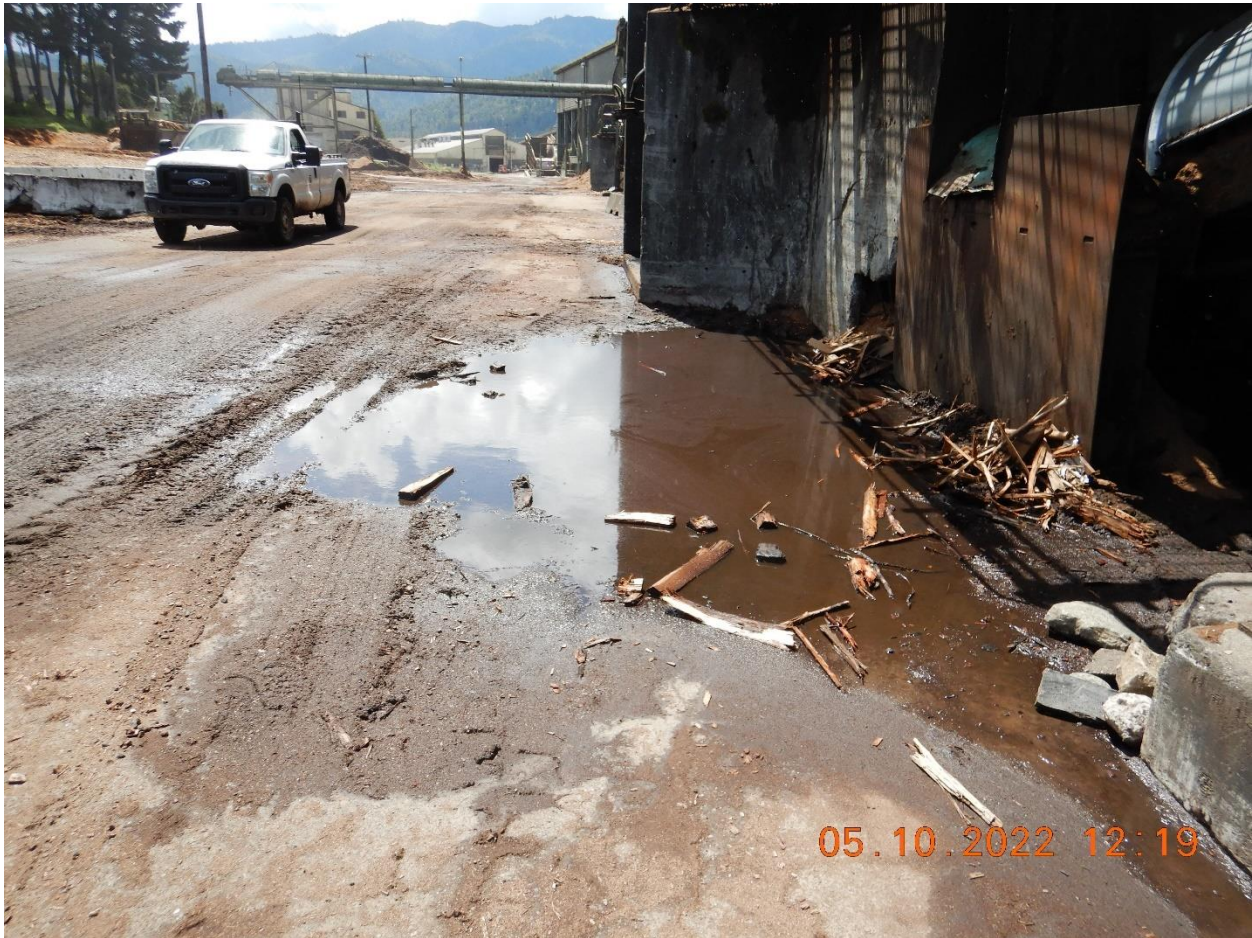
Picture 20c: Looking South at sawmill yard in Drainage Area 2. Standing stormwater in this area was dark brown and had a visible oil sheen. Picture taken by Farzad Kasmaei.
