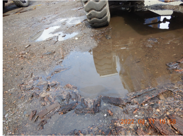
Pictures 2d and 2e: Industrial equipment and associated oil sheen in drainage area 1 exposed to rain. This area is covered with many inches debris, mud, wood fiber and directly adjacent to unprotected storm drain inlets. No housekeeping BMPs or inlet protection BMPs are present. Picture taken by Heaven Moore.
