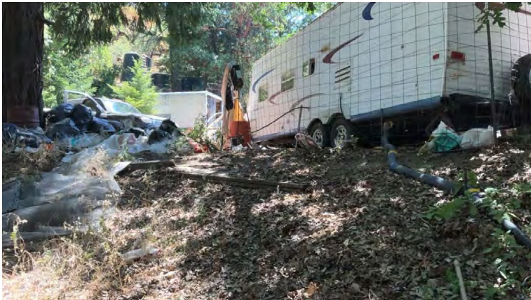
Figure 7. Point 13. RV with waste line into drainage swale.
