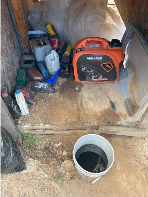
Photo 3: Petroleum products in open buckets with small spill on wood board.
