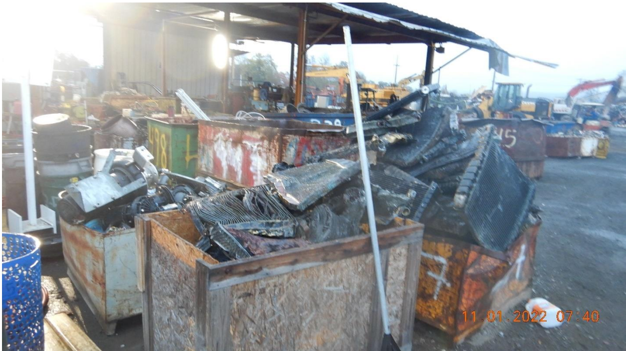
Picture 8 – View of radiators and other scrap metals all stored inappropriately in the non-sealed and rusty bins exposed to rain. Picture taken by Farzad Kasmaei.
