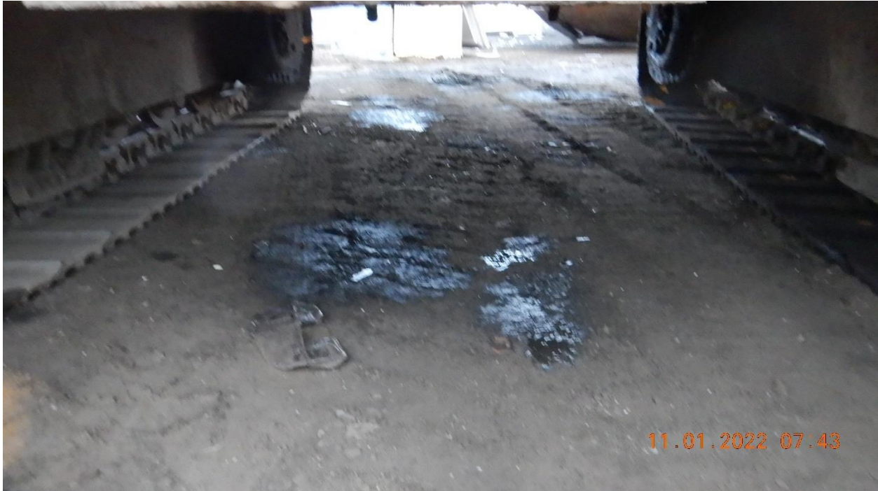
Picture 12 – View of hydrocarbon leaks from a dozer that was parked within the facility's yard. Drip pans are not used to capture any potential spills. Picture taken by Farzad Kasmaei.
