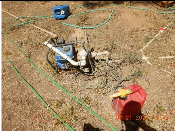
Photo 7 – uncontained pump and gasoline tank around WQ5
