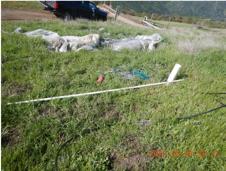
Figure 6—Looking southwest at WQ2. A white pipe protrudes up from the ground in the middle of the image and an orange submersible pump is visible to the left of the white pipe. Plastic sheeting covers holes used to collect water in the top back of the image.
