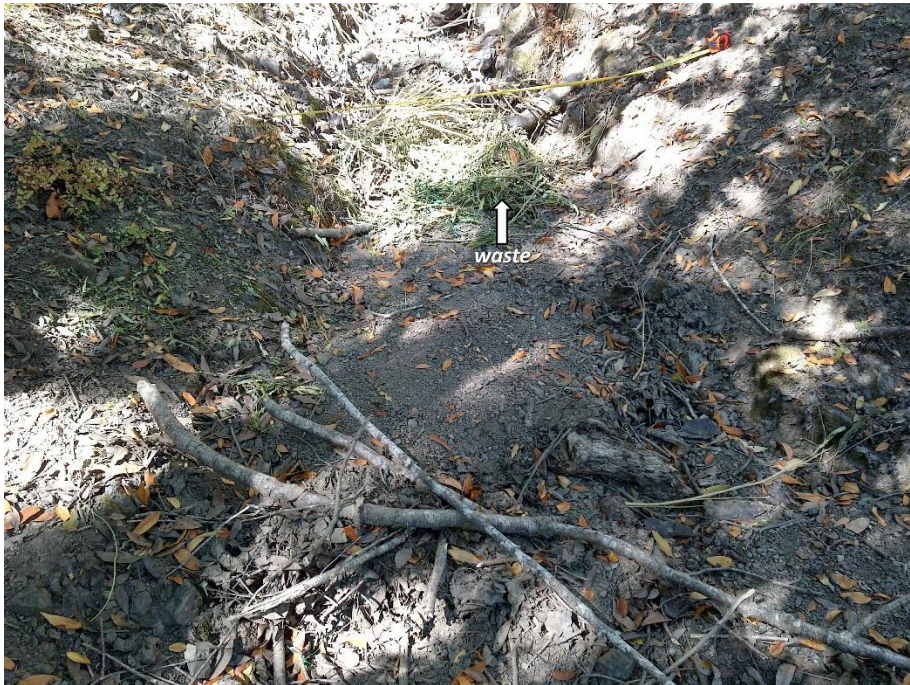
Figure 8—Photo, looking upstream, showing waste cannabis plants, marked by an arrow, in watercourse at WQ4. The report author measured the local channel width of 4.5 feet with the tape measure visible in the top of the image.
