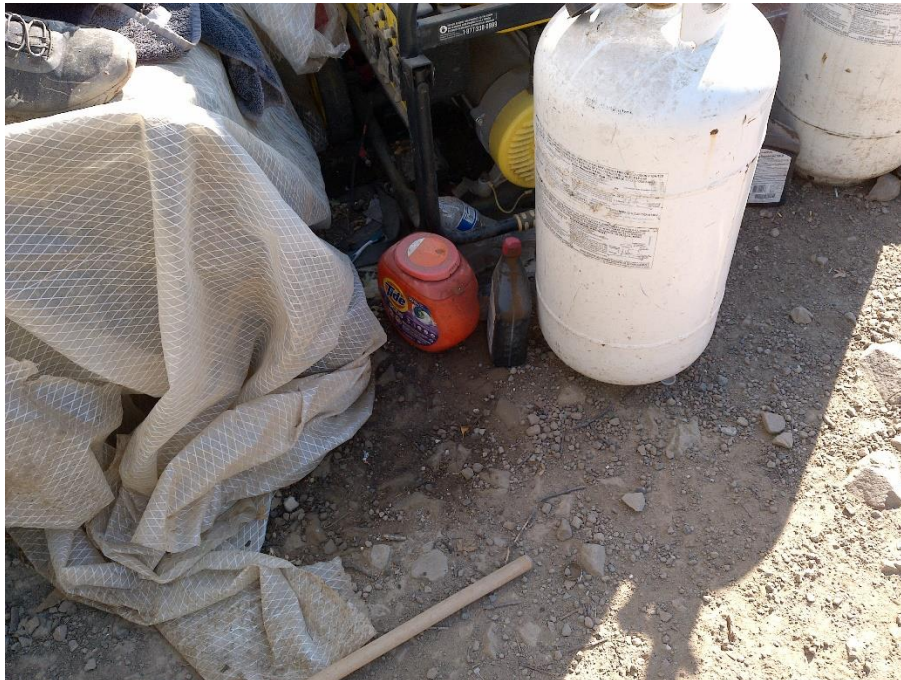
Figure 9—Generator and motor oil stored at WQ5 without secondary containment. The earth in the vicinity of the petroleum product storage area is darker than surrounding areas.
