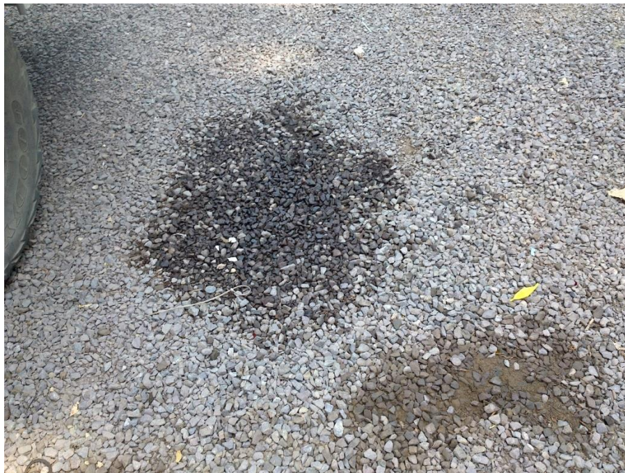
Figure 13—Patches of oil-stained ground at WQ4. The earthen ground is covered by a layer of permeable rock.
