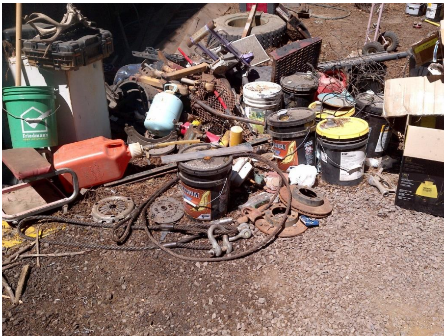
Figure 12—Picture of petroleum products in five-gallon buckets without secondary containment ground in the vicinity of WQ4. A thin layer of gravel covers the earthen ground. The ground to the left of the image is darker in color apparently from spilled petroleum products.
