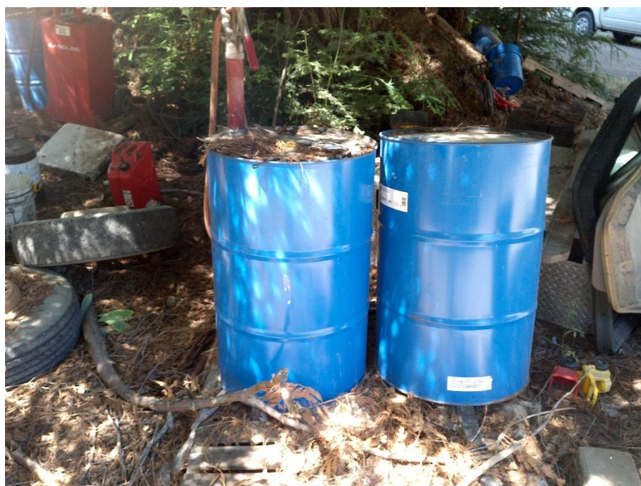
Figure 14—Two of many 55-gallon drums without secondary containment in the vicinity of WQ4. A pipe and hose are connected to the drum in the middle left suggesting that there are intended fluid transfers at its current location.
