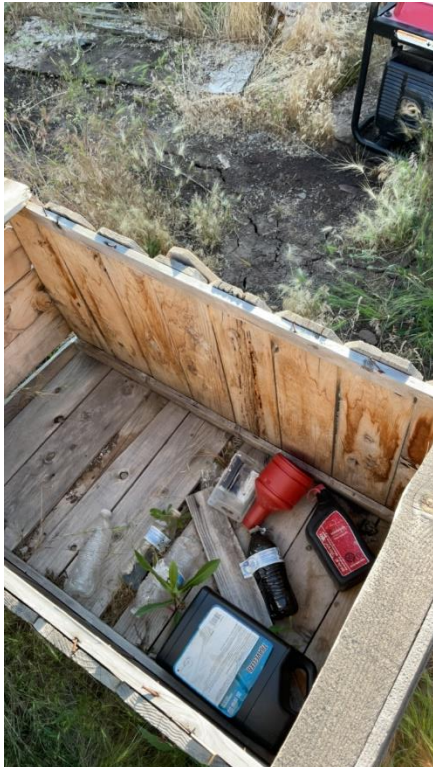
Photo 6: Petroleum product stored in water bottle. Fuel spill near edge of generator.
