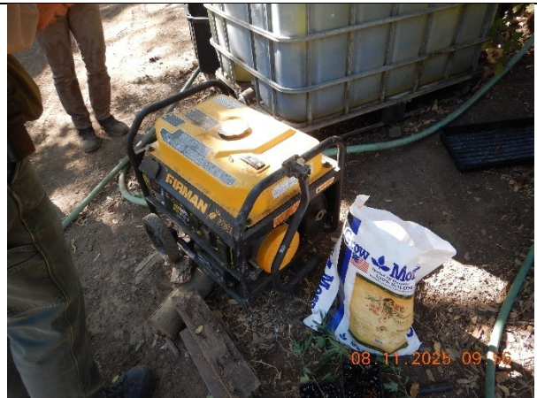
Photo 44 A generator and fertilizer without secondary containment or cover near WQ7
