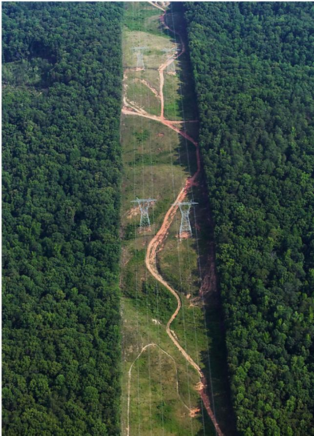
Image 1: high voltage transmission line and cleared corridor. Source: Google Images
