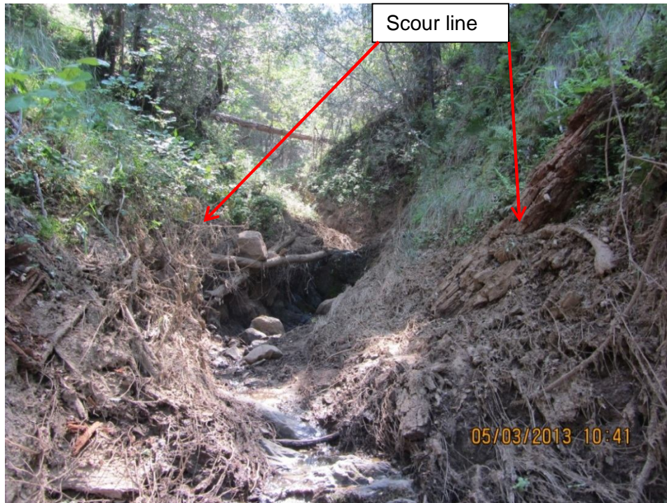
Image 3, May 3, 2013, this is taken upstream from the M8 Road crossing. Note the scour line: this shows the depth of flow during the discharge from the bladder failure. This is likely a perennial stream
