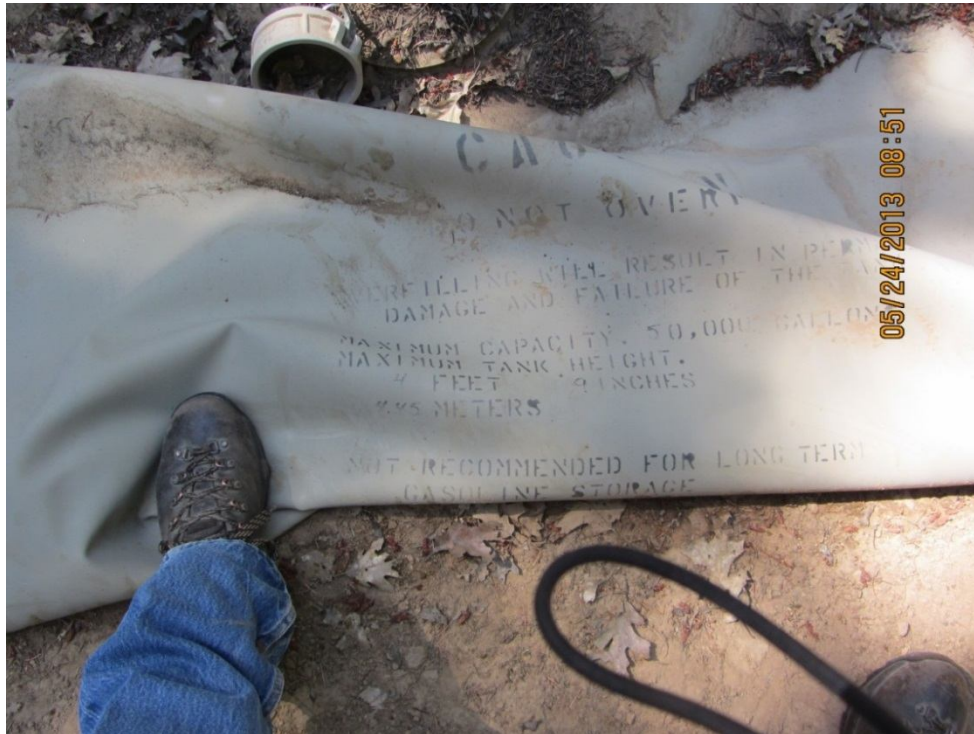
Image 9, May 24, 2013, water bladder label, which indicates it has a maximum capacity of 50,000 gallons. The bladder is designed for use with fuels, and not recommended for long term use.
