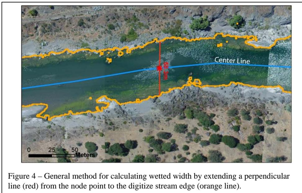
Figure 4 – General method for calculating wetted width by extending a perpendicular line (red) from the node point to the digitize stream edge (orange line).
