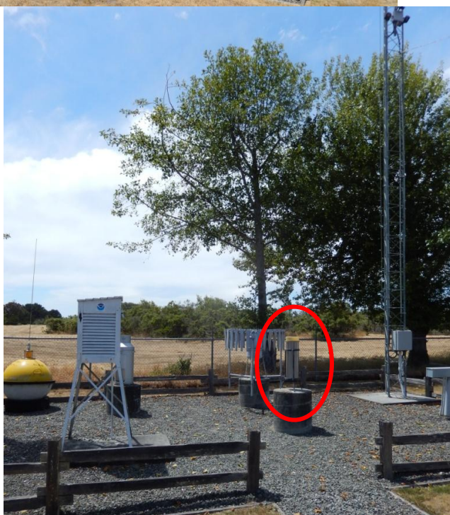
Figure 1. Pictures of the weather station outside of the NOAA office in Eureka taken in summer 2013. The official Eureka rain gage is located just behind the rain gage with the Alter shield, so it is to the left of the wooden temperature shelter in a), and to the right in b). This shows how the adjacent trees are almost certainly having an increasing effect on the official rainfall measurements.
