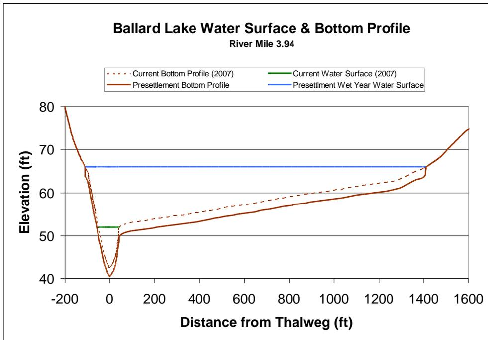
Figure 30. Water Surface and Bottom Profiles at Laguna River Mile 3.94
