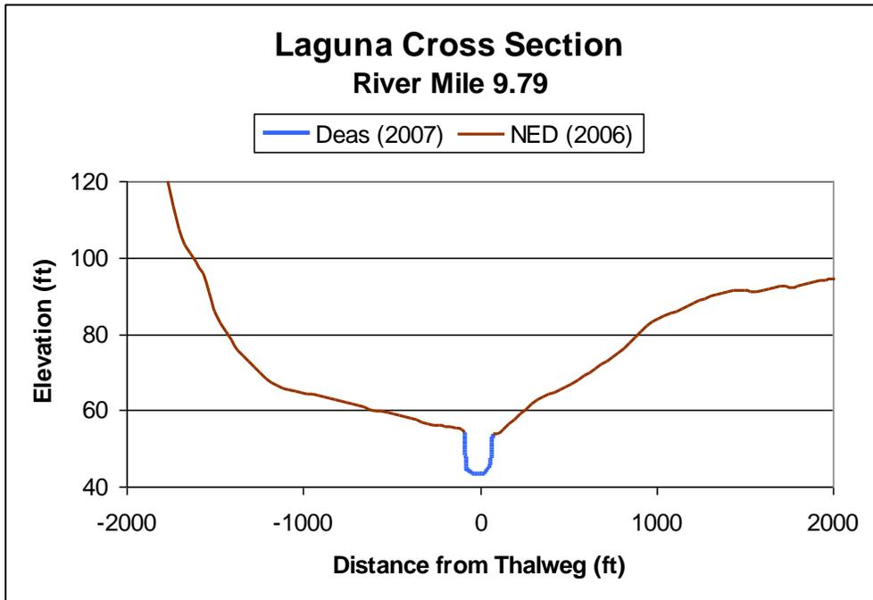
Figure 23. Elevation Profile at Laguna River Mile 9.79
