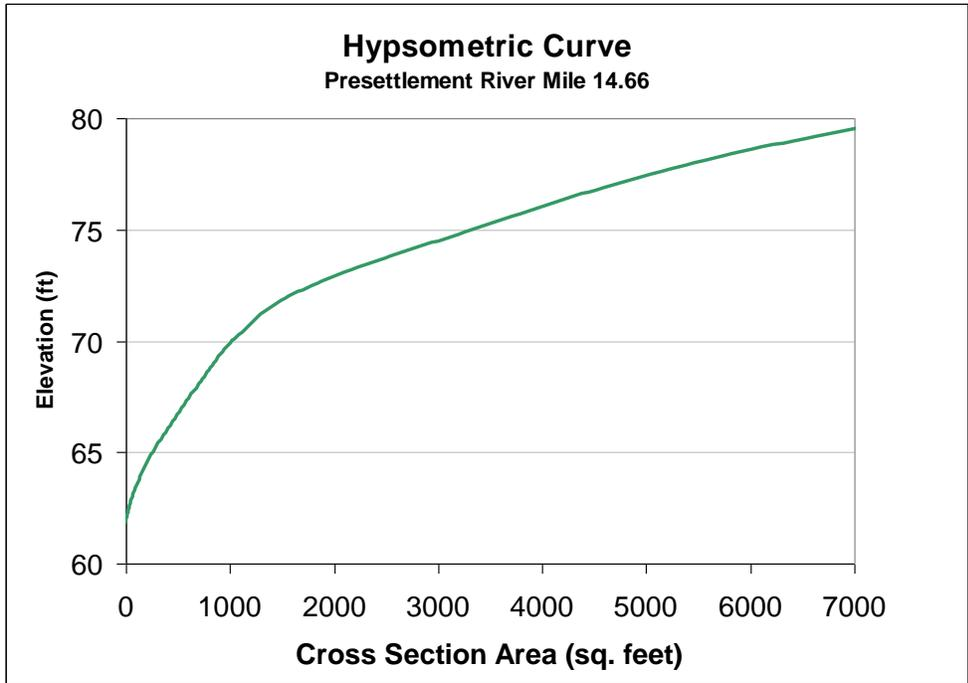
Figure 49. Hypsometric Curve at Pre-settlement River Mile 14.66
