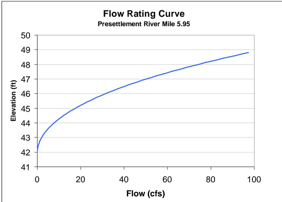
Figure 53. Flow Rating Curve at Pre-settlement River Mile 5.95
