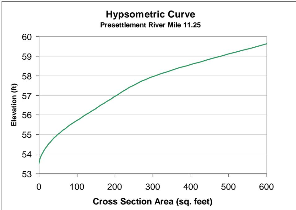
Figure 47. Hypsometric Curve at Pre-settlement River Mile 11.25
