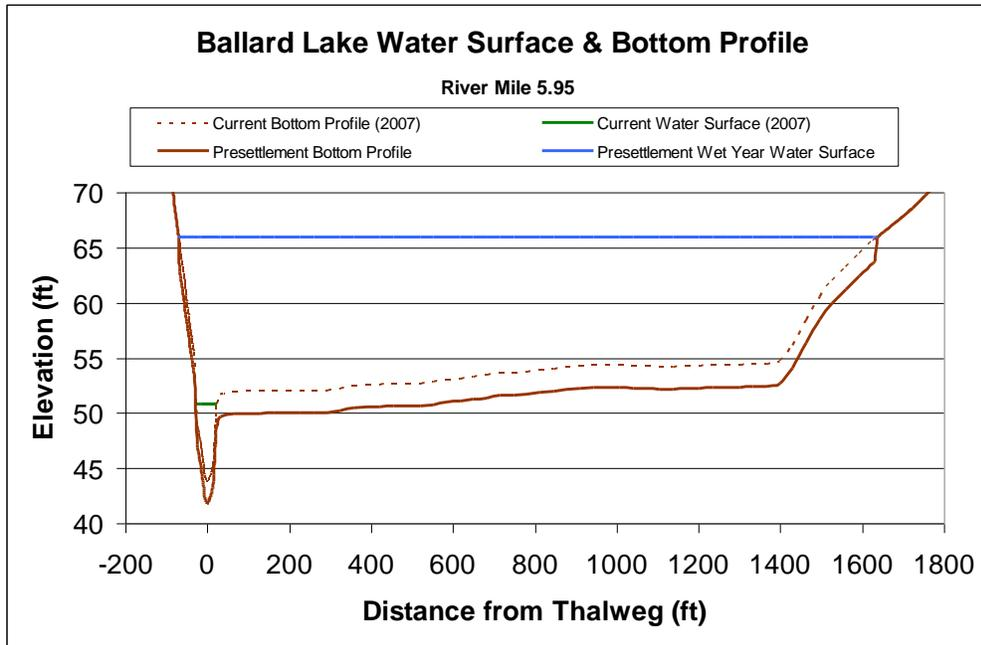
Figure 31. Water Surface and Bottom Profiles at Laguna River Mile 5.95
