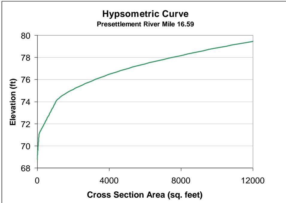
Figure 51. Hypsometric Curve at Pre-settlement River Mile 16.59
