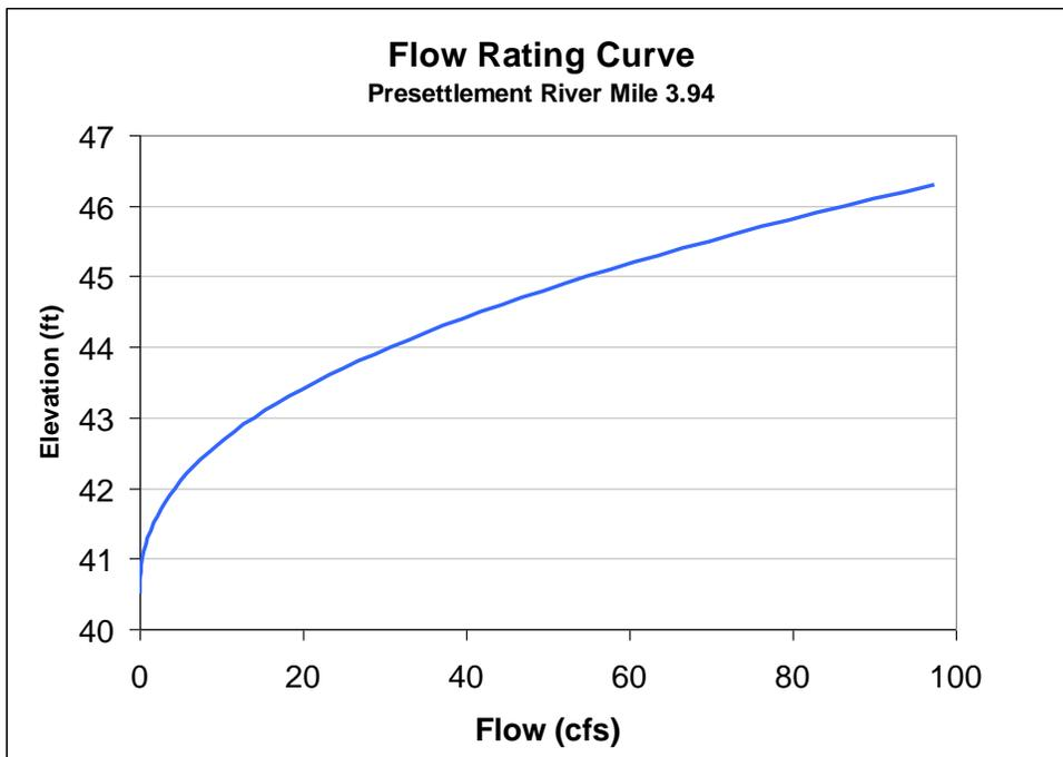
Figure 52. Flow Rating Curve at Pre-settlement River Mile 3.94
