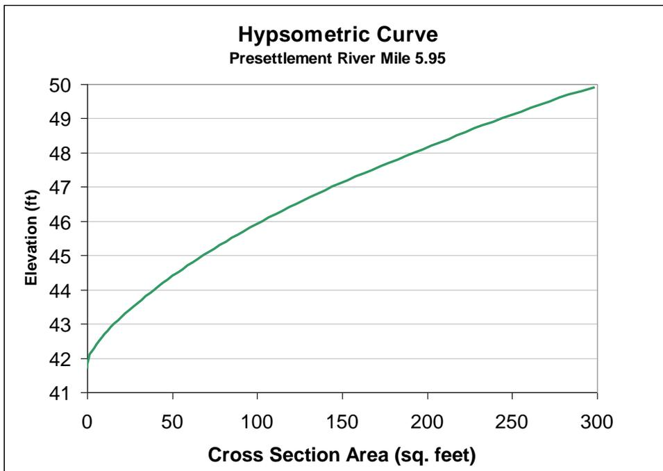
Figure 42. Hypsometric Curve at Pre-settlement River Mile 5.95
