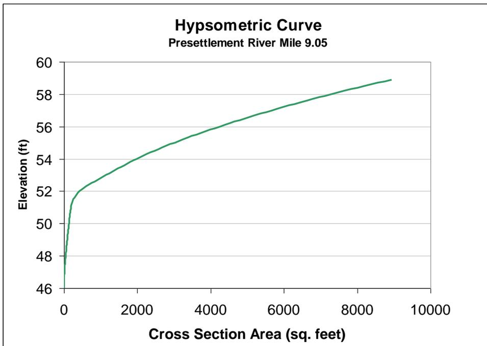
Figure 44. Hypsometric Curve at Pre-settlement River Mile 9.05
