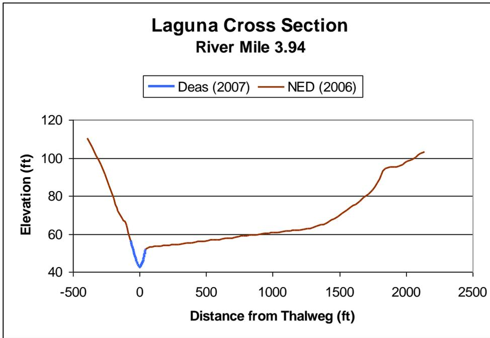
Figure 19. Elevation Profile at Laguna River Mile 3.94
