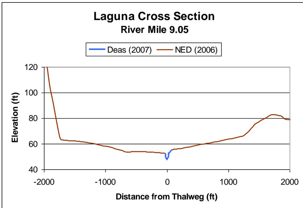
Figure 22. Elevation Profile at Laguna River Mile 9.05
