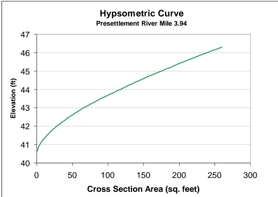
Figure 41. Hypsometric Curve at Pre-settlement River Mile 3.94
