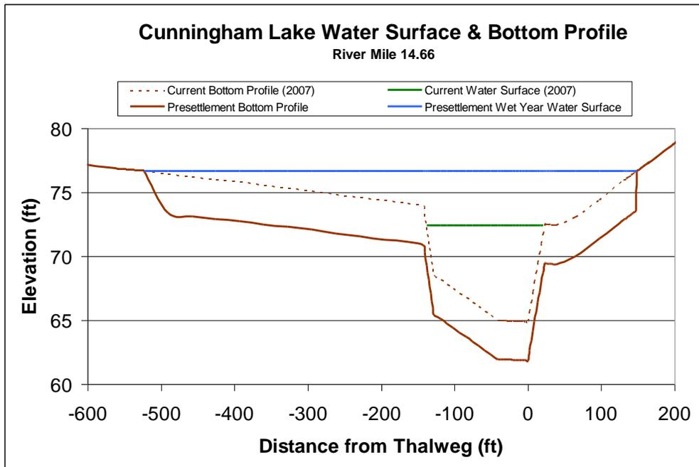
Figure 38. Water Surface and Bottom Profiles at Laguna River Mile 14.66
