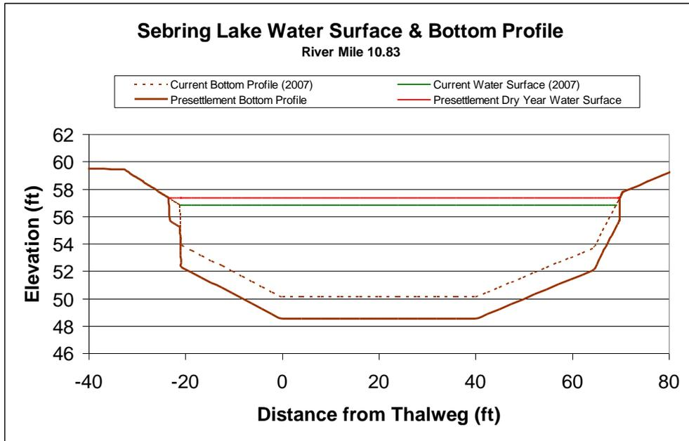
Figure 35. Water Surface and Bottom Profiles at Laguna River Mile 10.83
