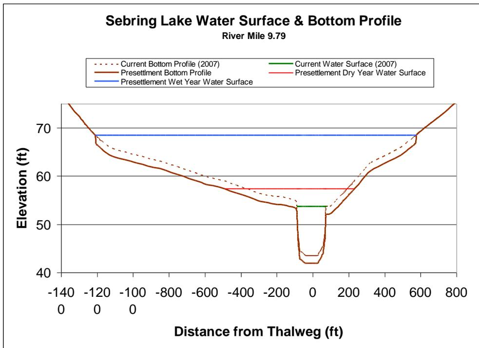
Figure 34. Water Surface and Bottom Profiles at Laguna River Mile 9.79
