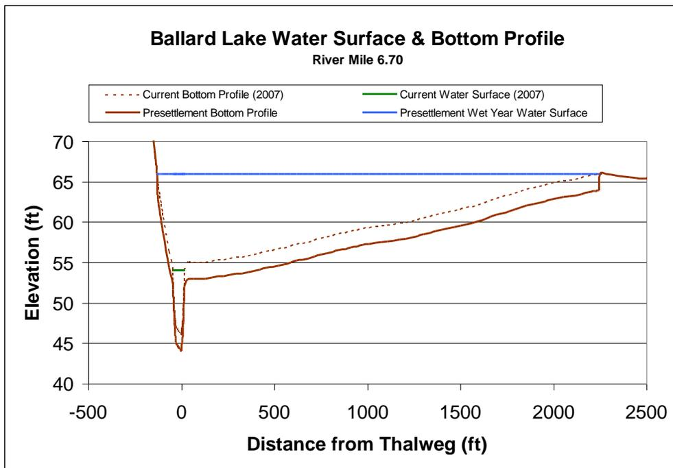
Figure 32. Water Surface and Bottom Profiles at Laguna River Mile 6.70
