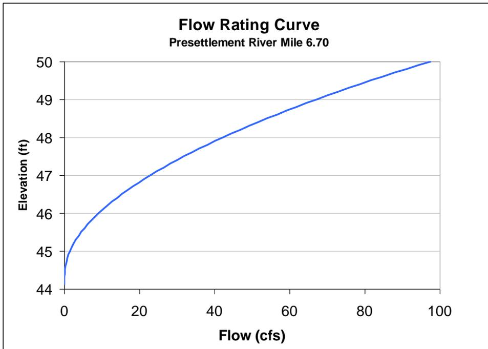
Figure 54. Flow Rating Curve at Pre-settlement River Mile 6.70
