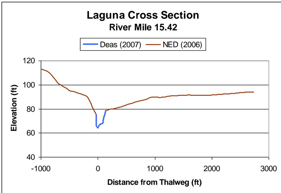
Figure 28. Elevation Profile at Laguna River Mile 15.42
