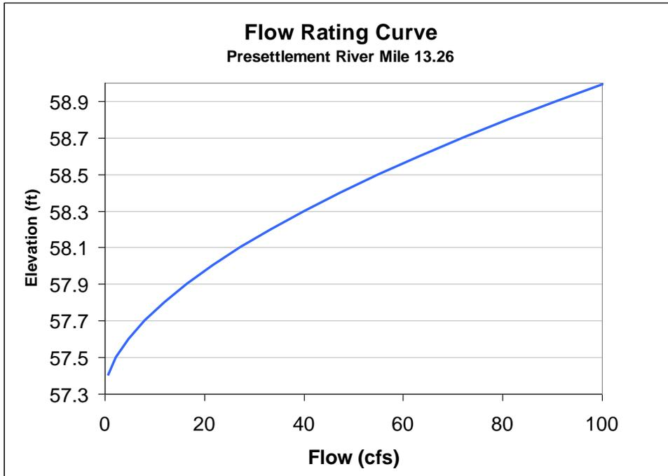
Figure 59. Flow Rating Curve at Pre-settlement River Mile 13.26
