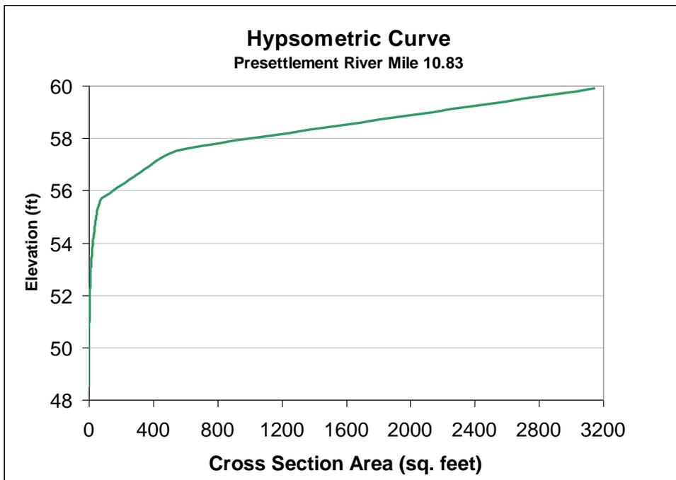
Figure 46. Hypsometric Curve at Pre-settlement River Mile 10.83
