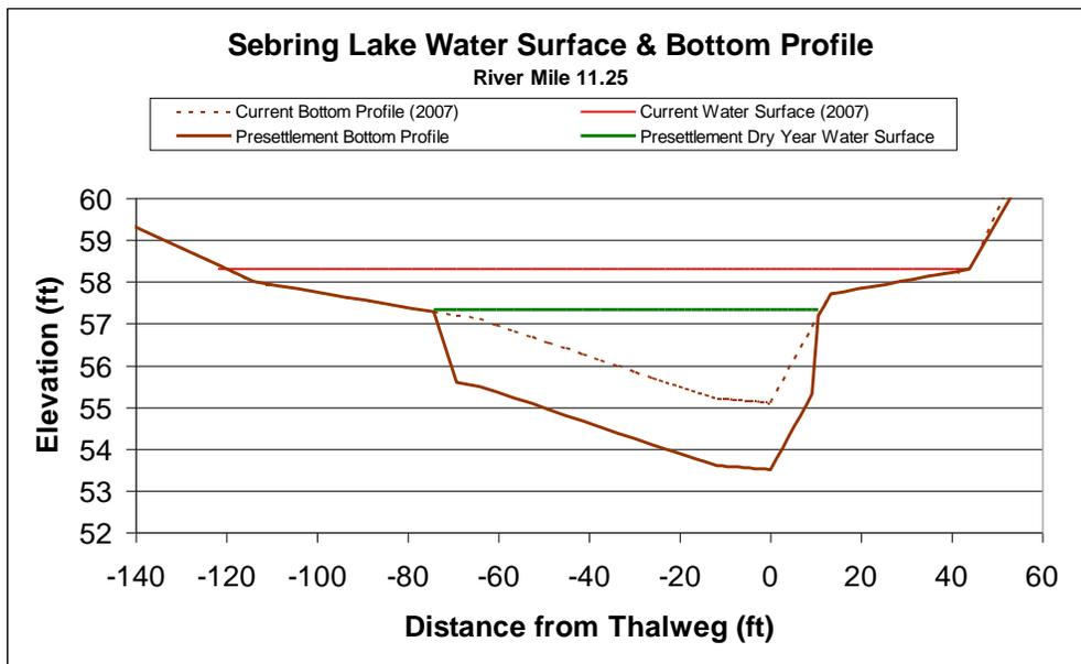
Figure 36. Water Surface and Bottom Profiles at Laguna River Mile 11.25
