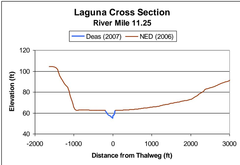
Figure 25. Elevation Profile at Laguna River Mile 11.25
