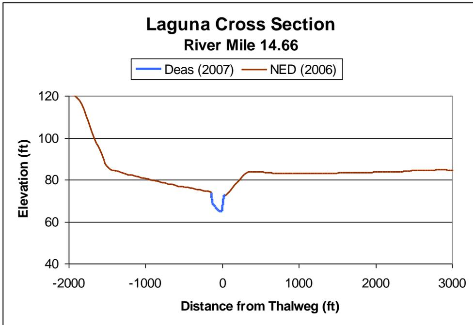
Figure 27. Elevation Profile at Laguna River Mile 14.66
