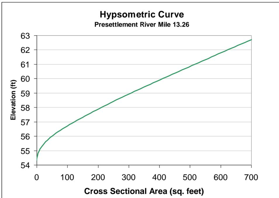
Figure 48. Hypsometric Curve at Pre-settlement River Mile 13.26
