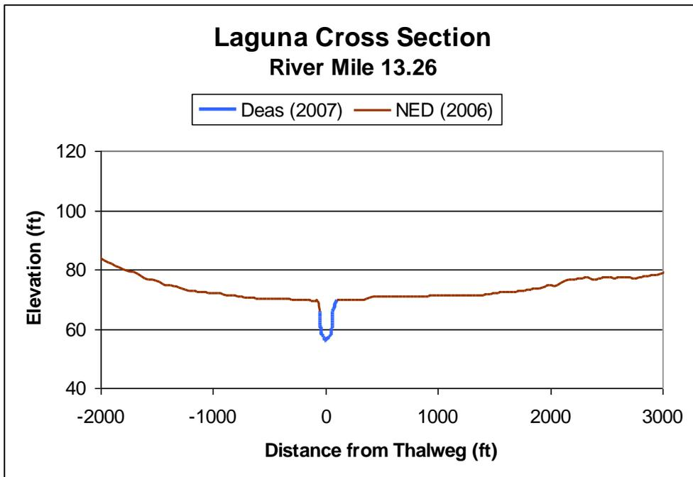
Figure 26. Elevation Profile at Laguna River Mile 13.26
