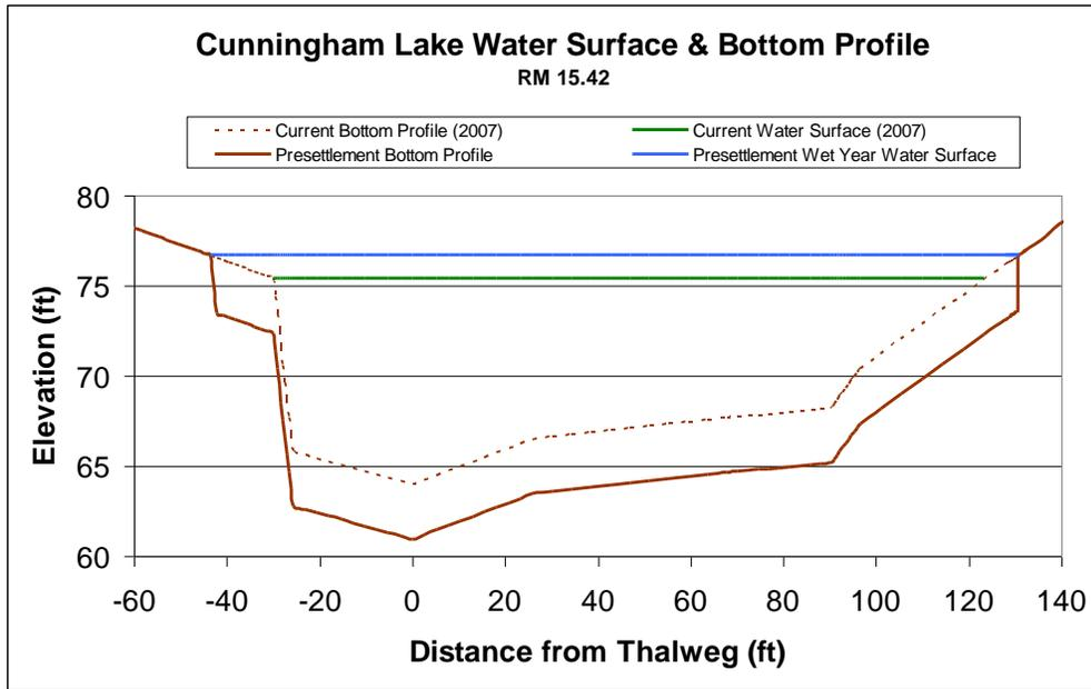
Figure 39. Water Surface and Bottom Profiles at Laguna River Mile 15.42
