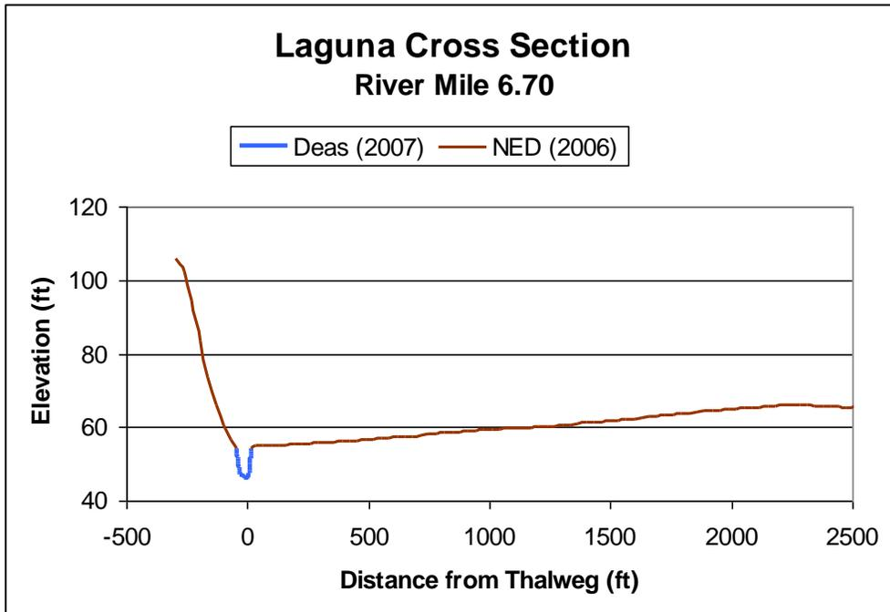
Figure 21. Elevation Profile at Laguna River Mile 6.70
