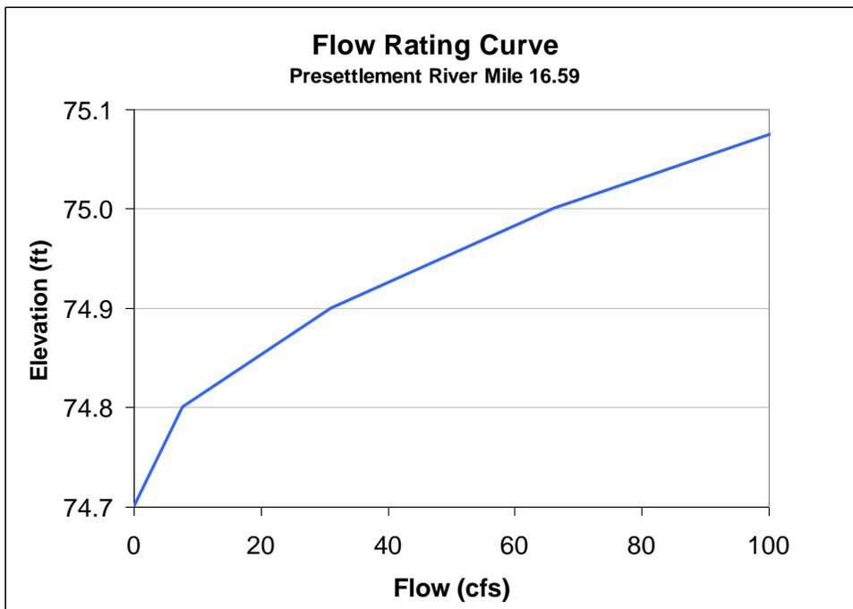
Figure 62. Flow Rating Curve at Pre-settlement River Mile 16.59
