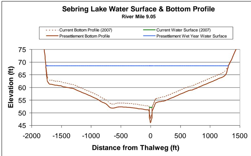
Figure 33. Water Surface and Bottom Profiles at Laguna River Mile 9.05
