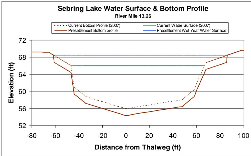
Figure 37. Water Surface and Bottom Profiles at Laguna River Mile 13.26
