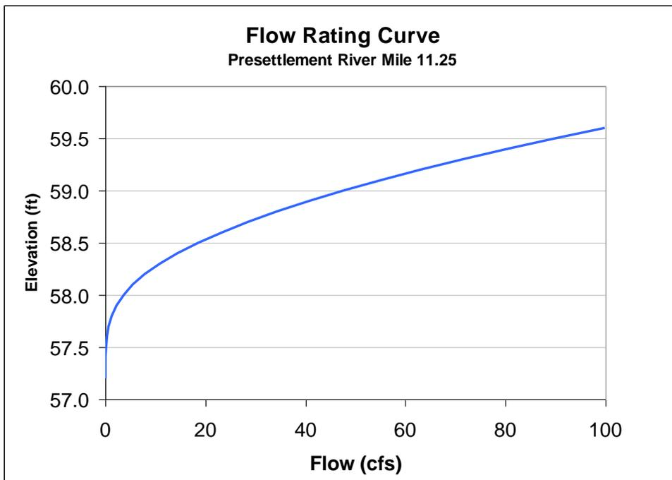
Figure 58. Flow Rating Curve at Pre-settlement River Mile 11.25
