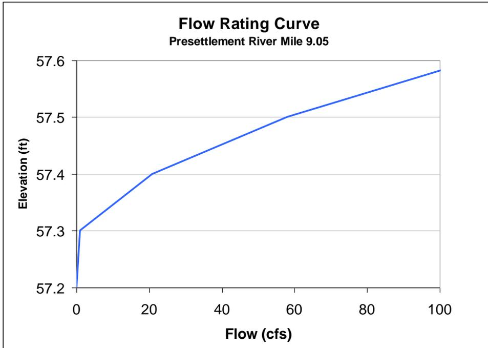
Figure 55. Flow Rating Curve at Pre-settlement River Mile 9.05
