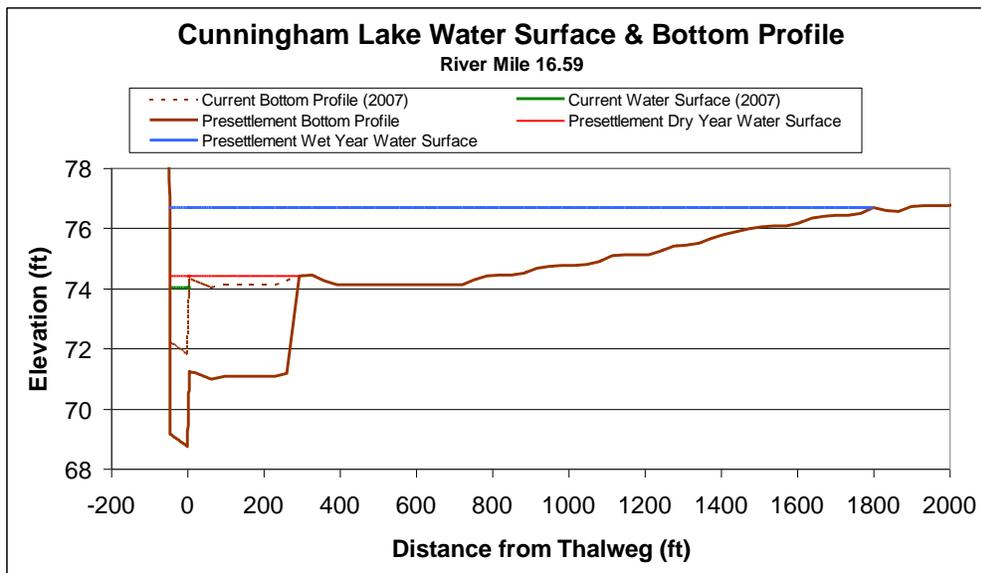
Figure 40. Water Surface and Bottom Profiles at Laguna River Mile 16.59
