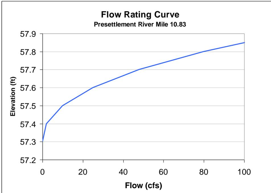
Figure 57. Flow Rating Curve at Pre-settlement River Mile 10.83
