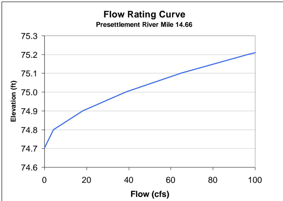
Figure 60. Flow Rating Curve at Pre-settlement River Mile 14.66
