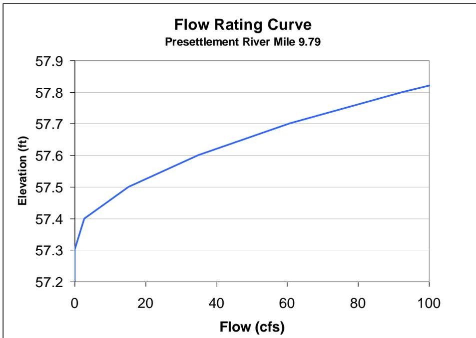
Figure 56. Flow Rating Curve at Pre-settlement River Mile 9.79
