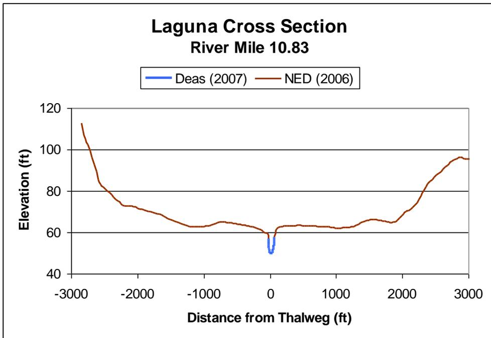
Figure 24. Elevation Profile at Laguna River Mile 10.83
