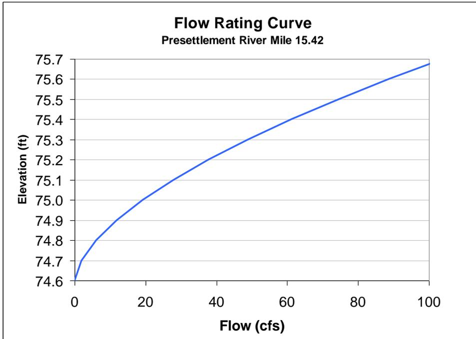
Figure 61. Flow Rating Curve at Pre-settlement River Mile 15.42
