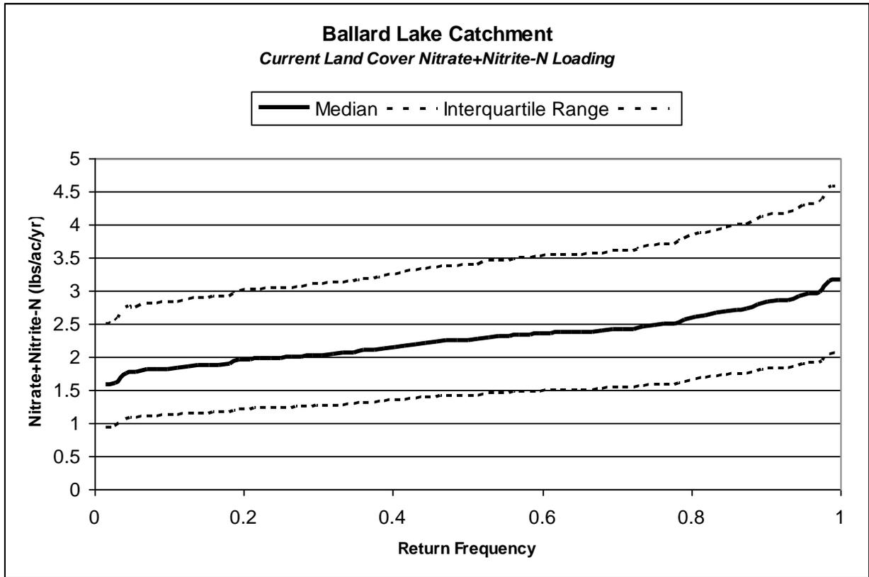
Figure 127. Current Ballard Lake Catchment Nitrate+Nitrite-N Load Duration Curve
