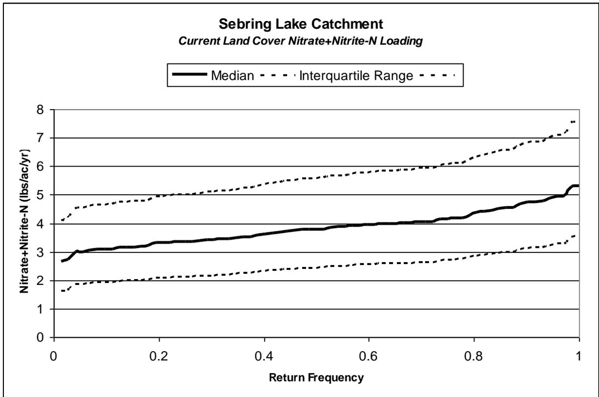
Figure 141. Current Sebring Lake Catchment Nitrate+Nitrite-N Load Duration Curve
