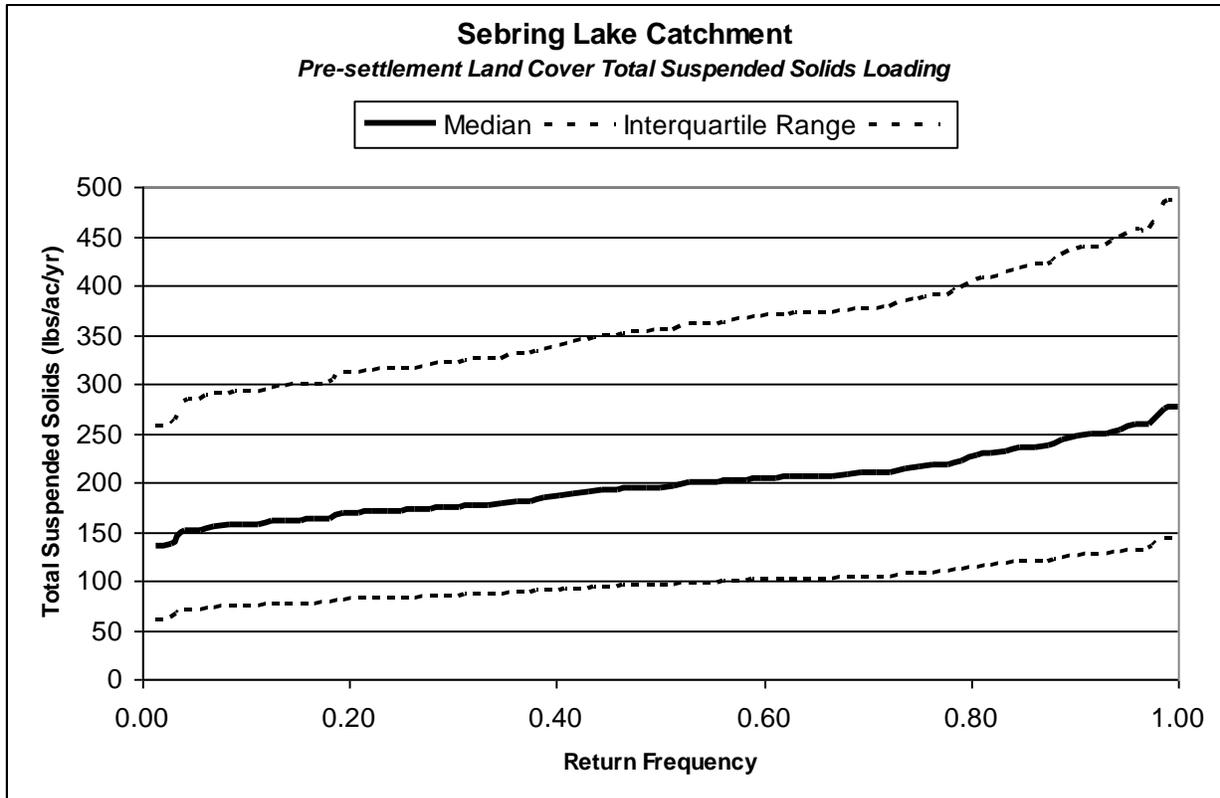
Figure 170. Pre-settlement Sebring Lake Catchment Total Suspended Solids Load Duration Curve
