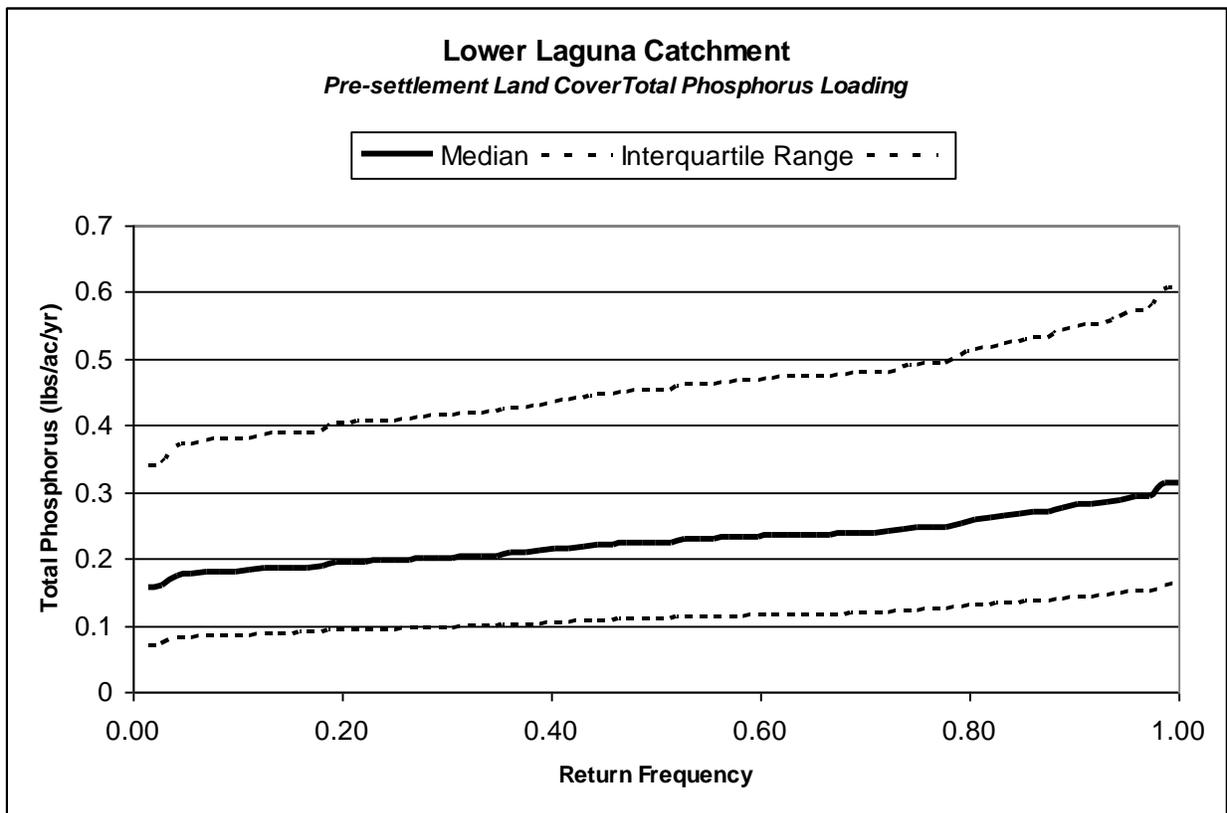
Figure 172. Pre-settlement Lower Laguna Catchment Total Phosphorus Load Duration Curve
