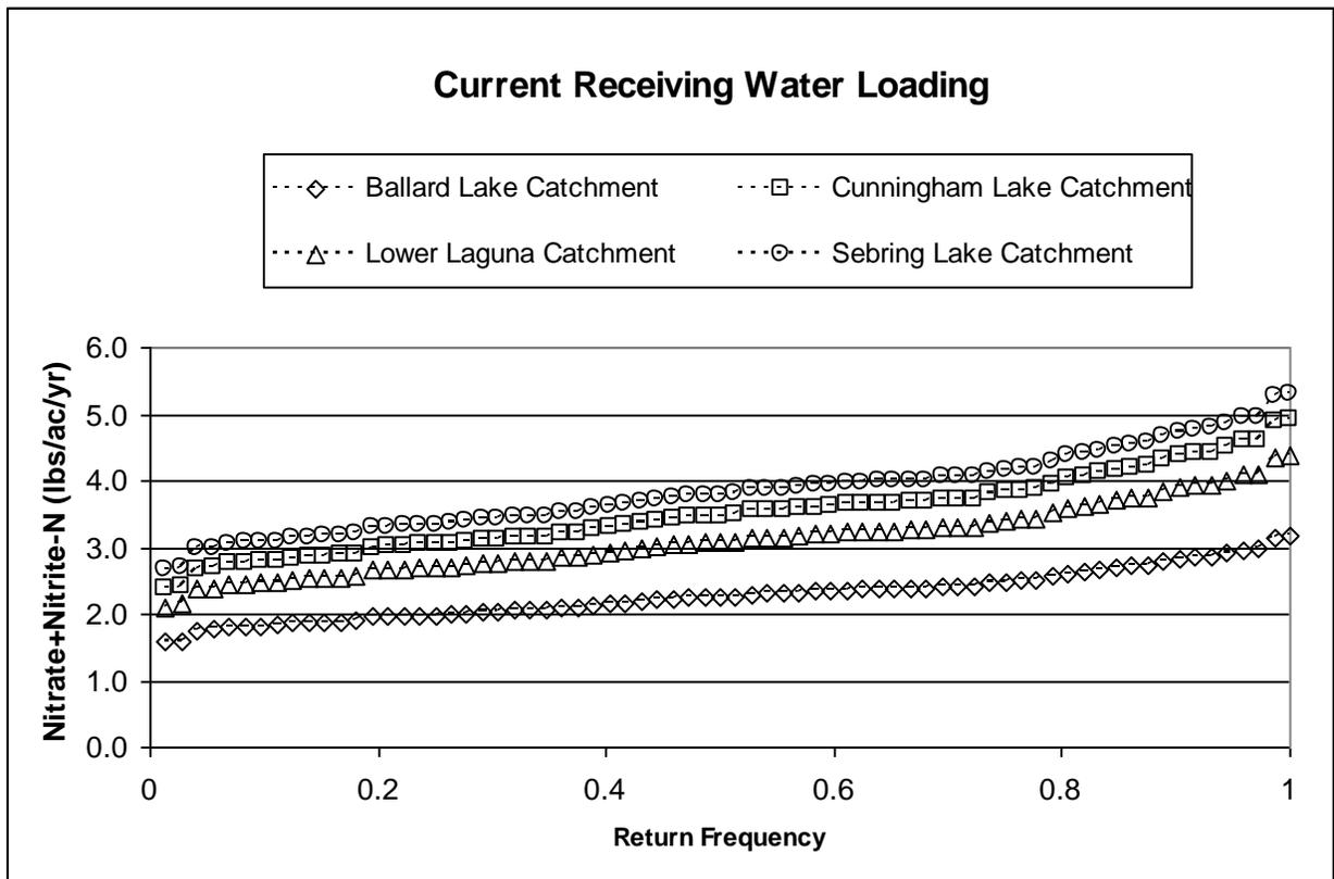
Figure 188. Comparison of Current Laguna Watershed Total Nitrate+Nitrite-N Load Duration Curves
