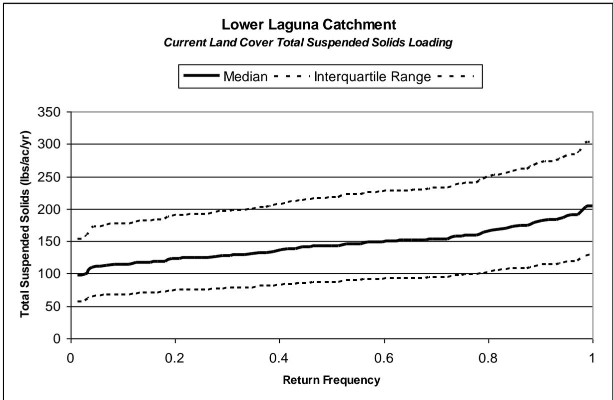
Figure 149. Current Lower Laguna Catchment Total Suspended Solids Load Duration Curve
