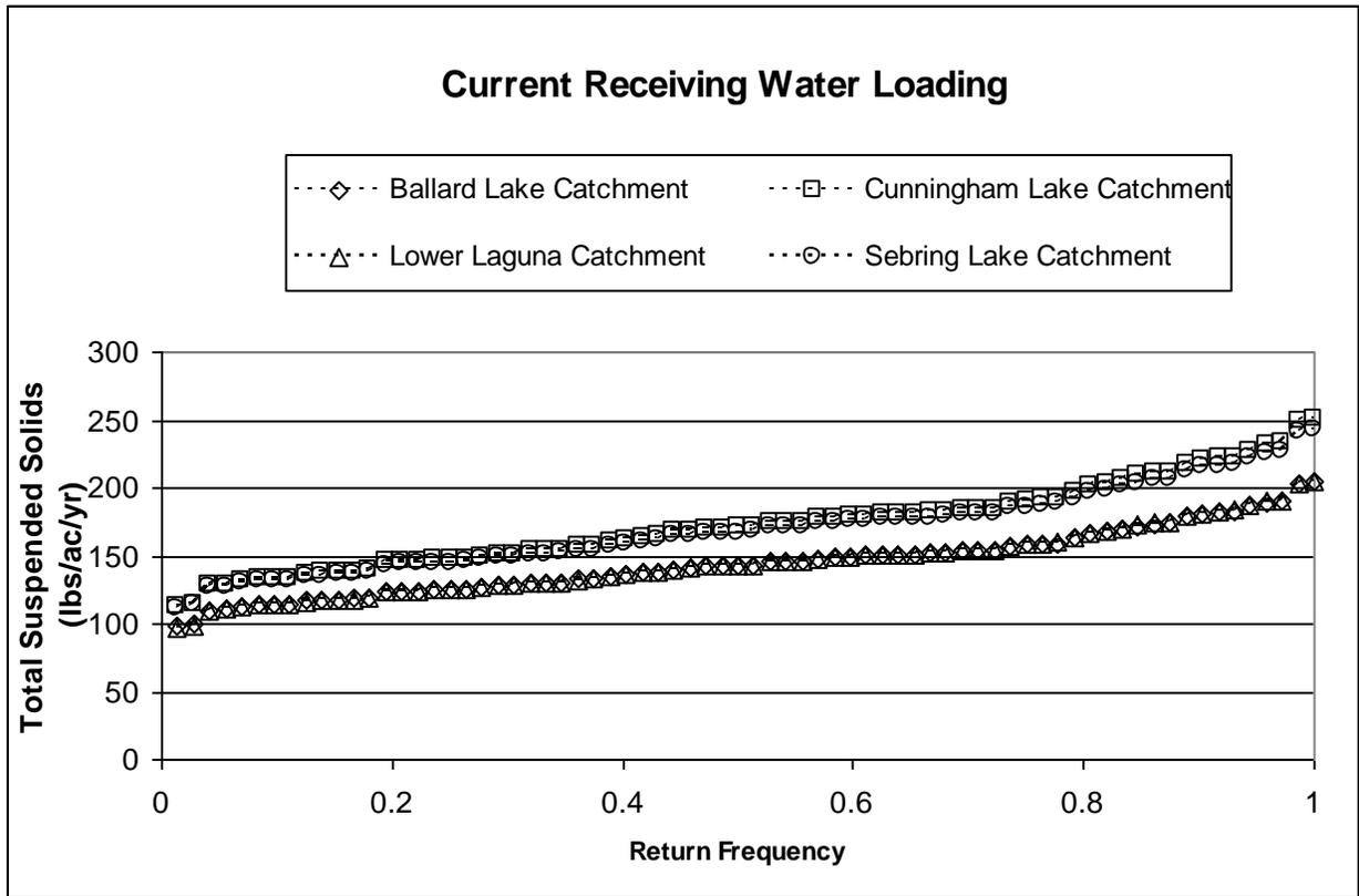
Figure 190. Comparison of Current Laguna Watershed Total Suspended Solids Load Duration Curves
