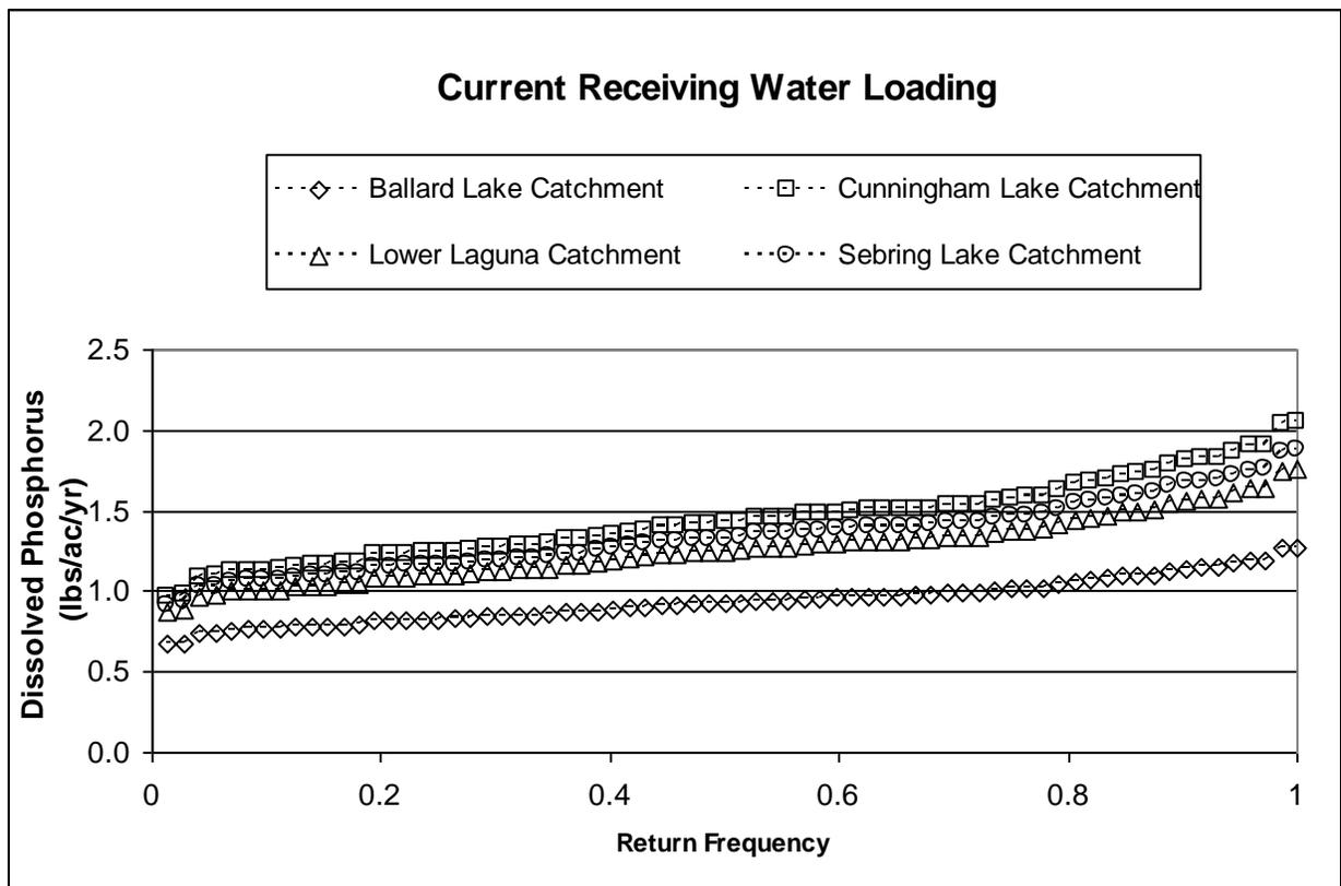
Figure 182. Comparison of Current Laguna Watershed Dissolved Phosphorus Load Duration Curves
