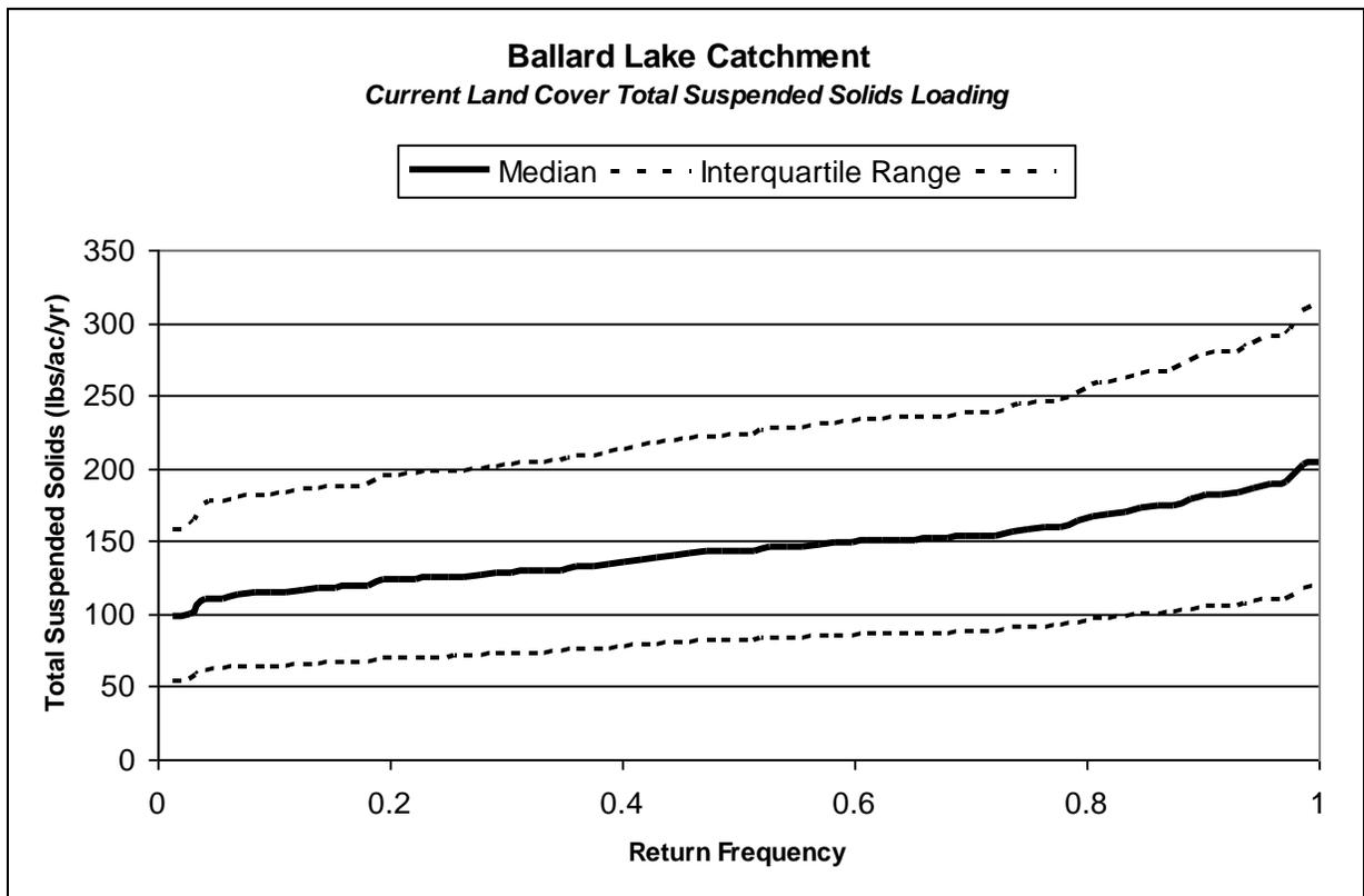
Figure 128. Current Ballard Lake Catchment Total Suspended Solids Load Duration Curve
