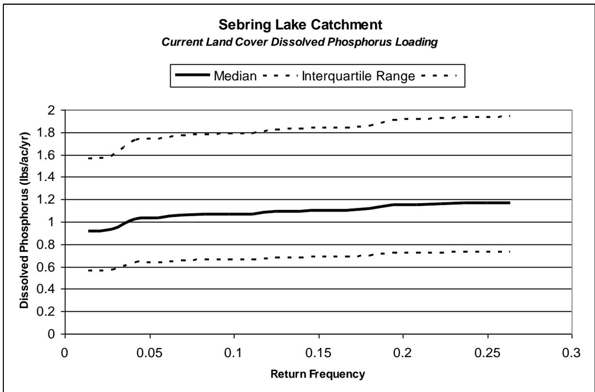
Figure 138. Current Sebring Lake Catchment Dissolved Phosphorus Load Duration Curve
