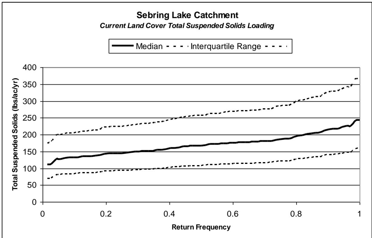
Figure 142. Current Sebring Lake Catchment Total Suspended Solids Load Duration Curve
