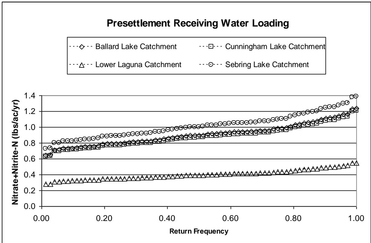
Figure 187. Comparison of Pre-Settlement Laguna Watershed Total Nitrate+Nitrite-N Load Duration Curves
