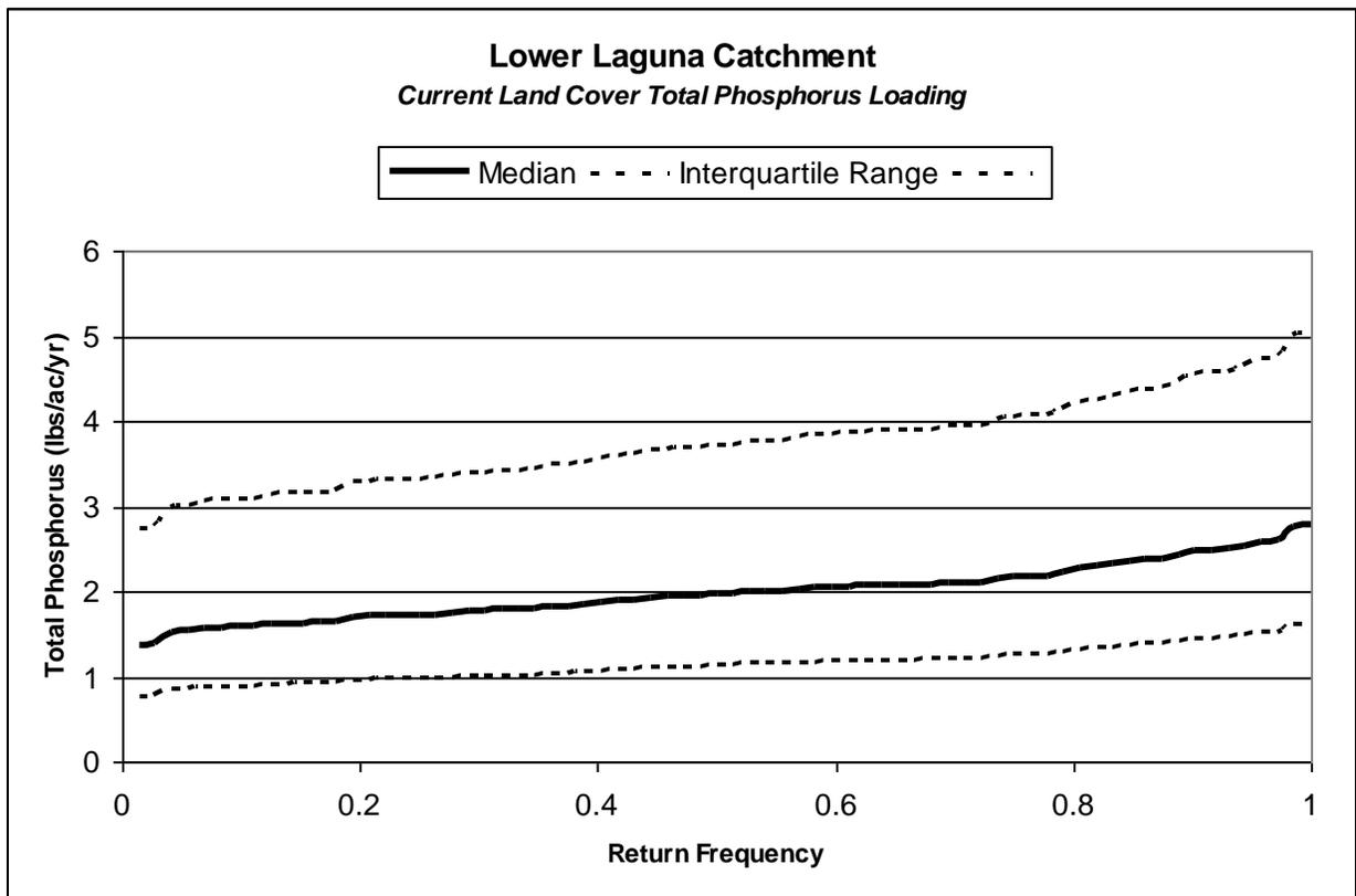
Figure 144. Current Lower Laguna Catchment Total Phosphorus Load Duration Curve
