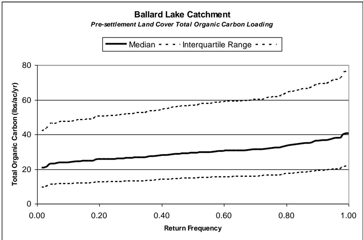
Figure 157. Pre-settlement Ballard Lake Catchment Total Organic Carbon Load Duration Curve
