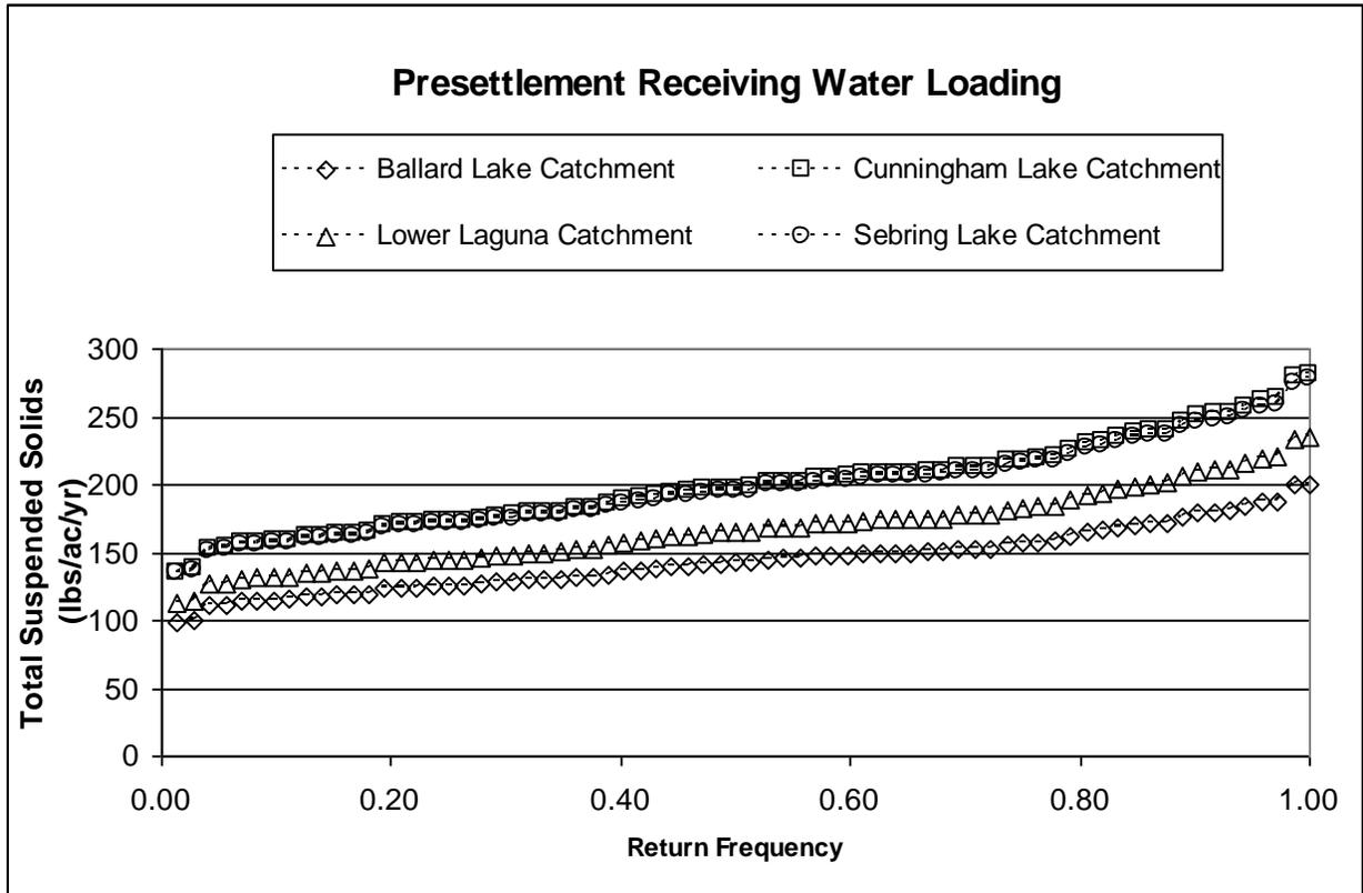
Figure 189. Comparison of Pre-Settlement Laguna Watershed Total Suspended Solids Load Duration Curves
