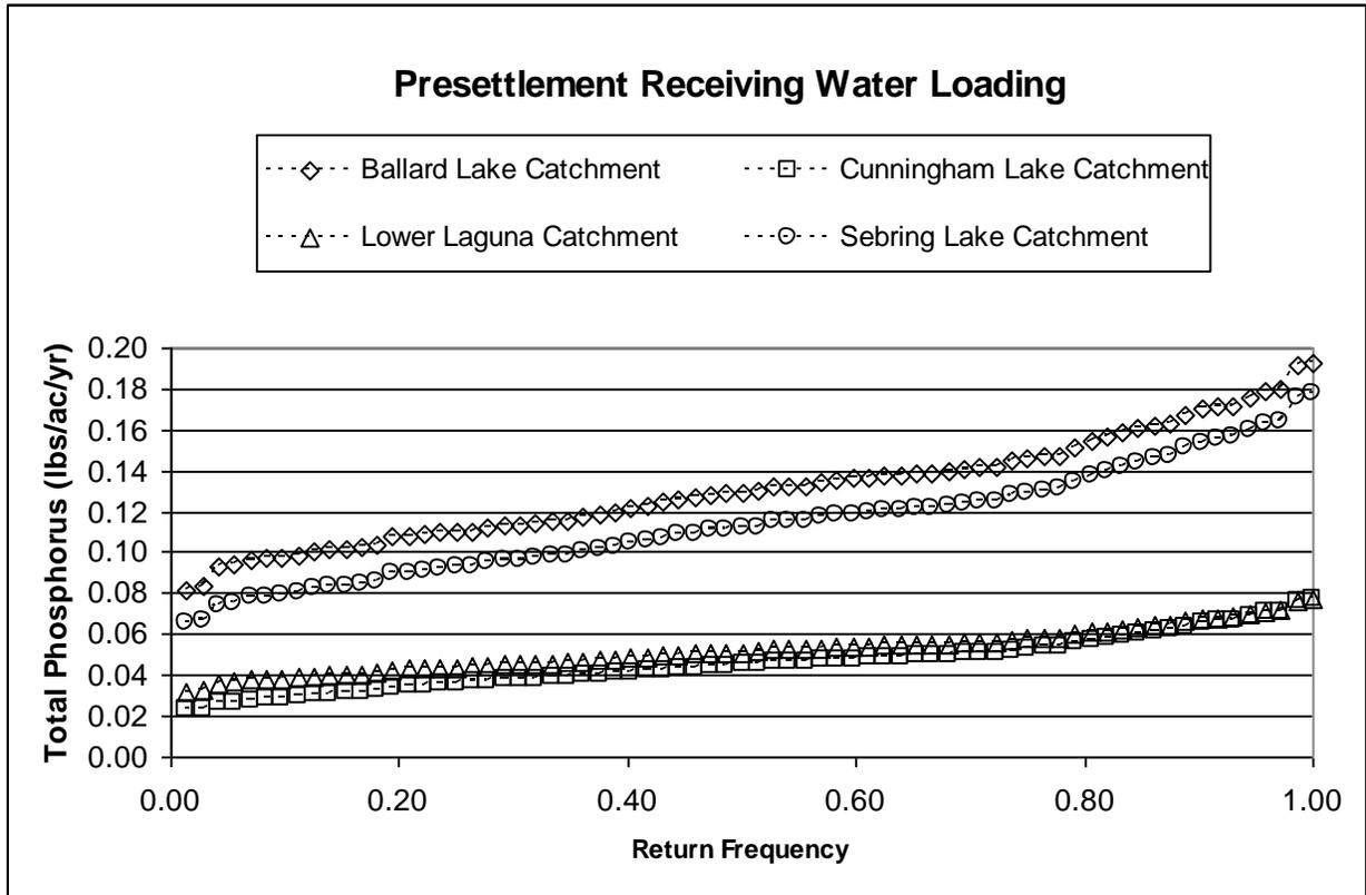
Figure 179. Comparison of Pre-Settlement Laguna Watershed Total Phosphorus Load Duration Curves
