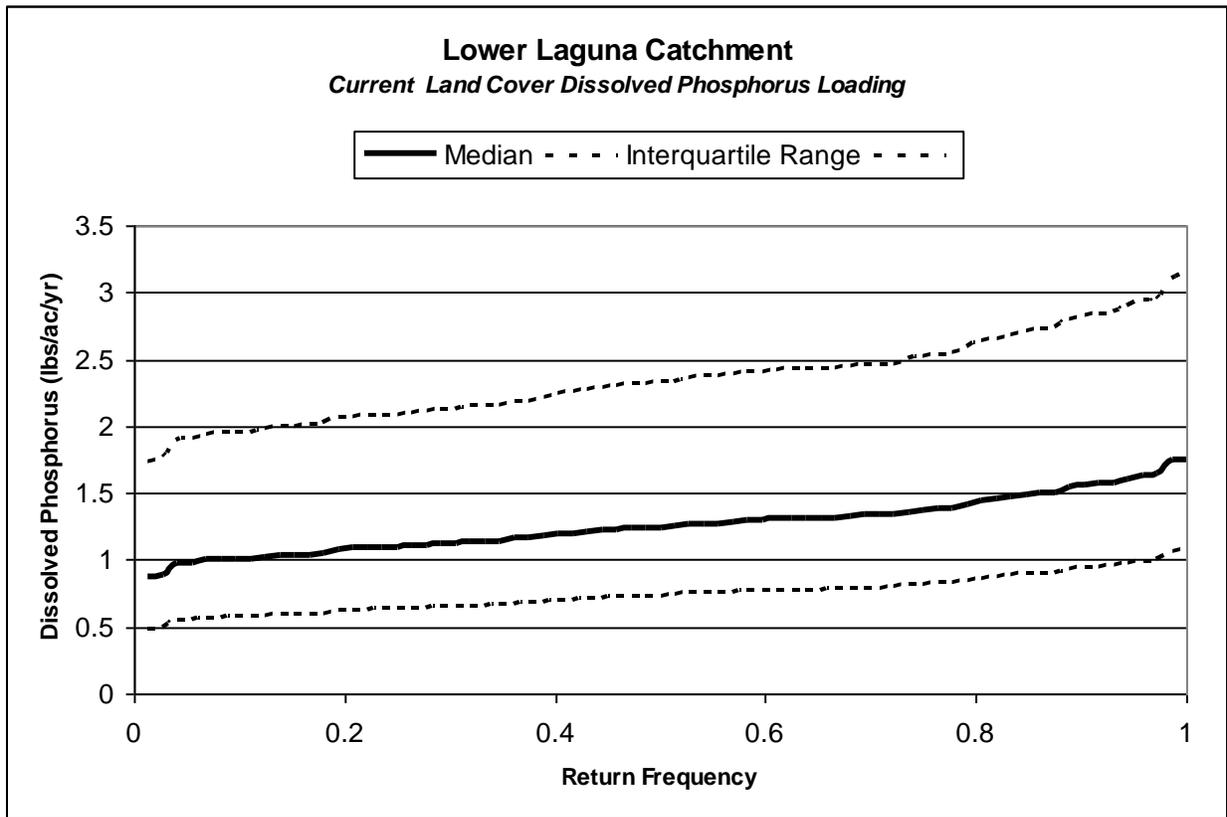
Figure 145. Current Lower Laguna Catchment Dissolved Phosphorus Load Duration Curve
