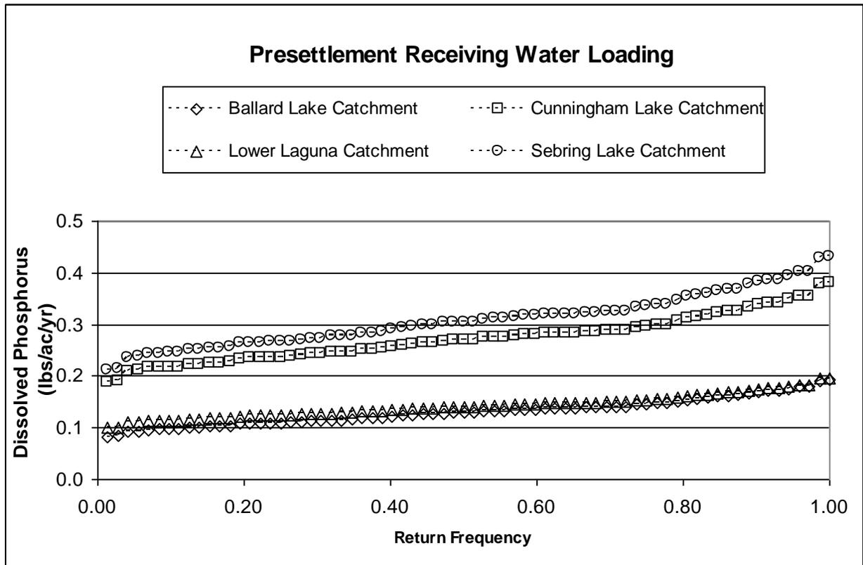
Figure 181. Comparison of Pre-Settlement Laguna Watershed Dissolved Phosphorus Load Duration Curves
