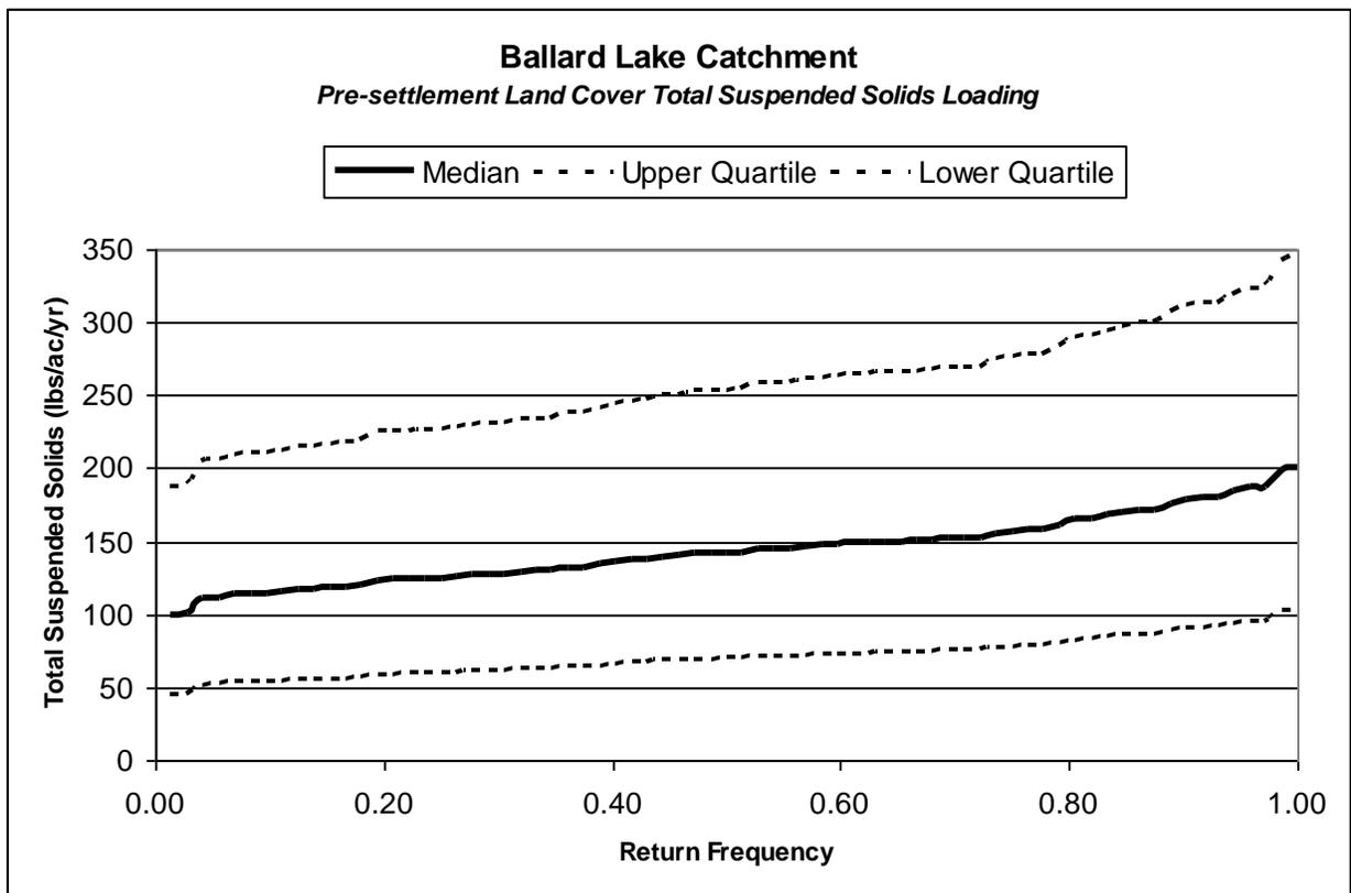
Figure 156. Pre-settlement Ballard Lake Catchment Total Suspended Solids Load Duration Curve
