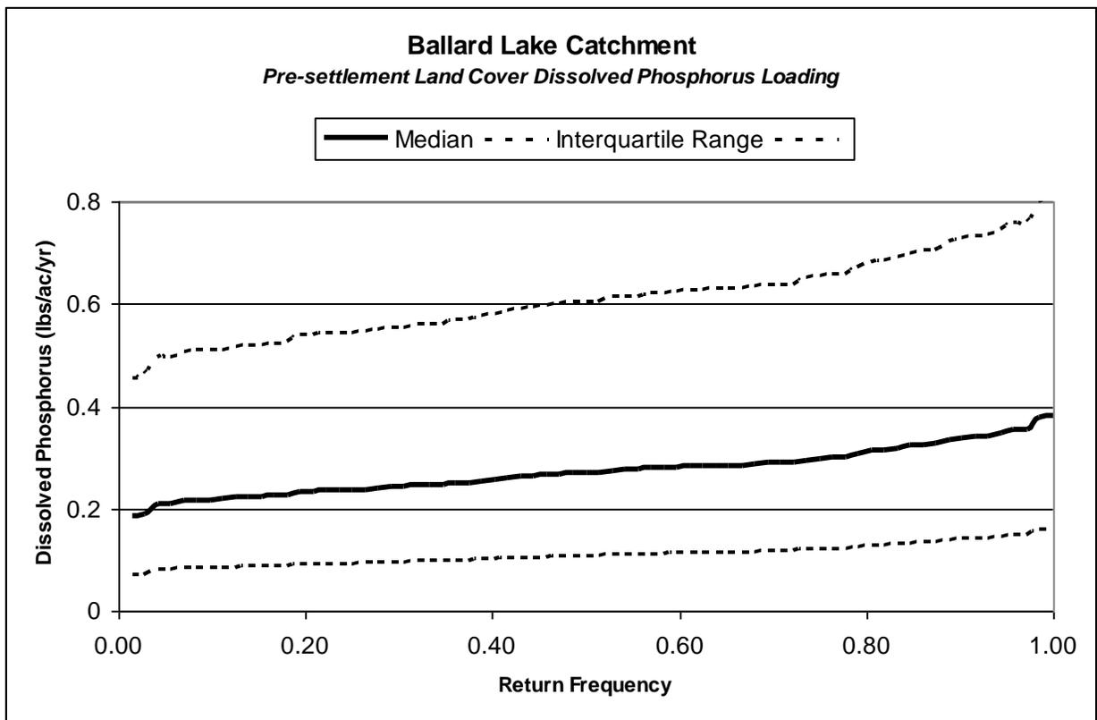
Figure 152. Pre-settlement Ballard Lake Catchment Dissolved Phosphorus Load Duration Curve
