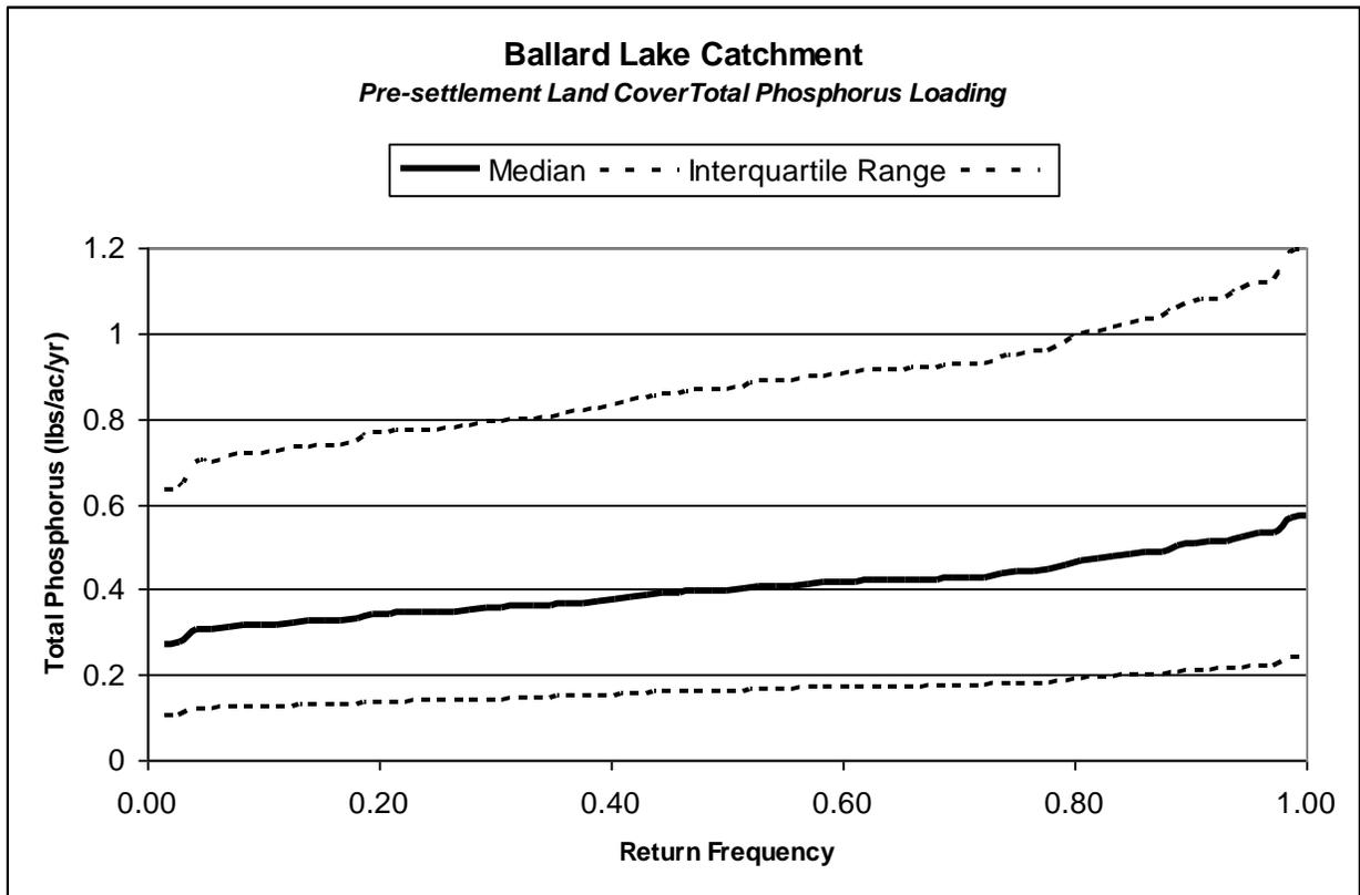
Figure 151. Pre-settlement Ballard Lake Catchment Total Phosphorus Load Duration Curve
