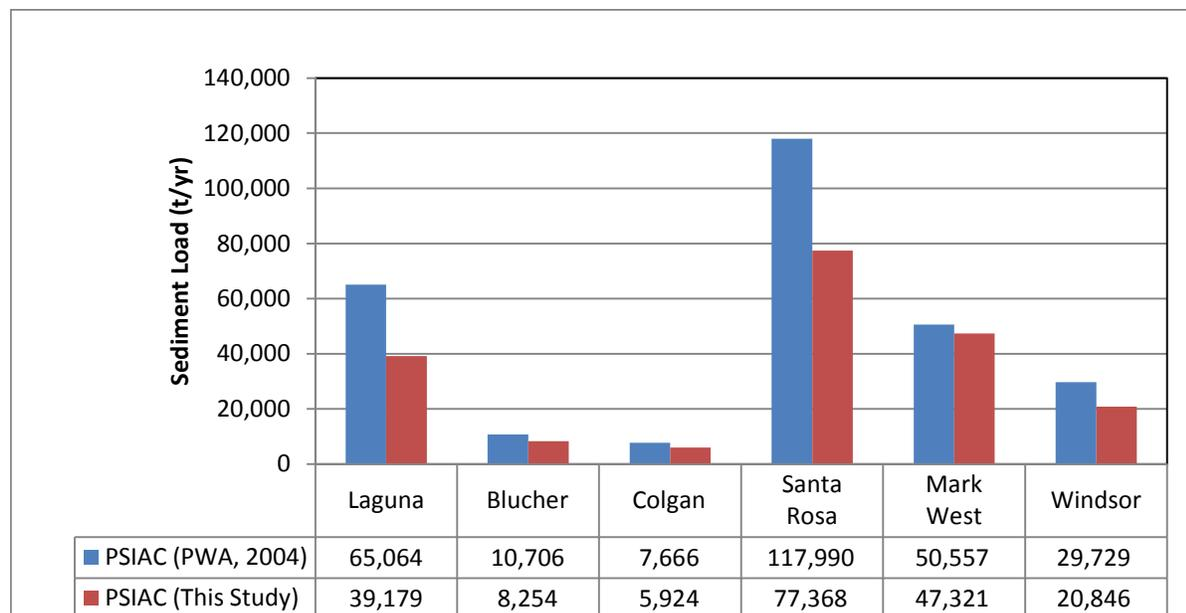
**Figure C-3. Comparison of PWA and Revised PSIAC Method Sediment Load Estimates for the Laguna de Santa Rosa Watershed (PWA Subbasins)**
