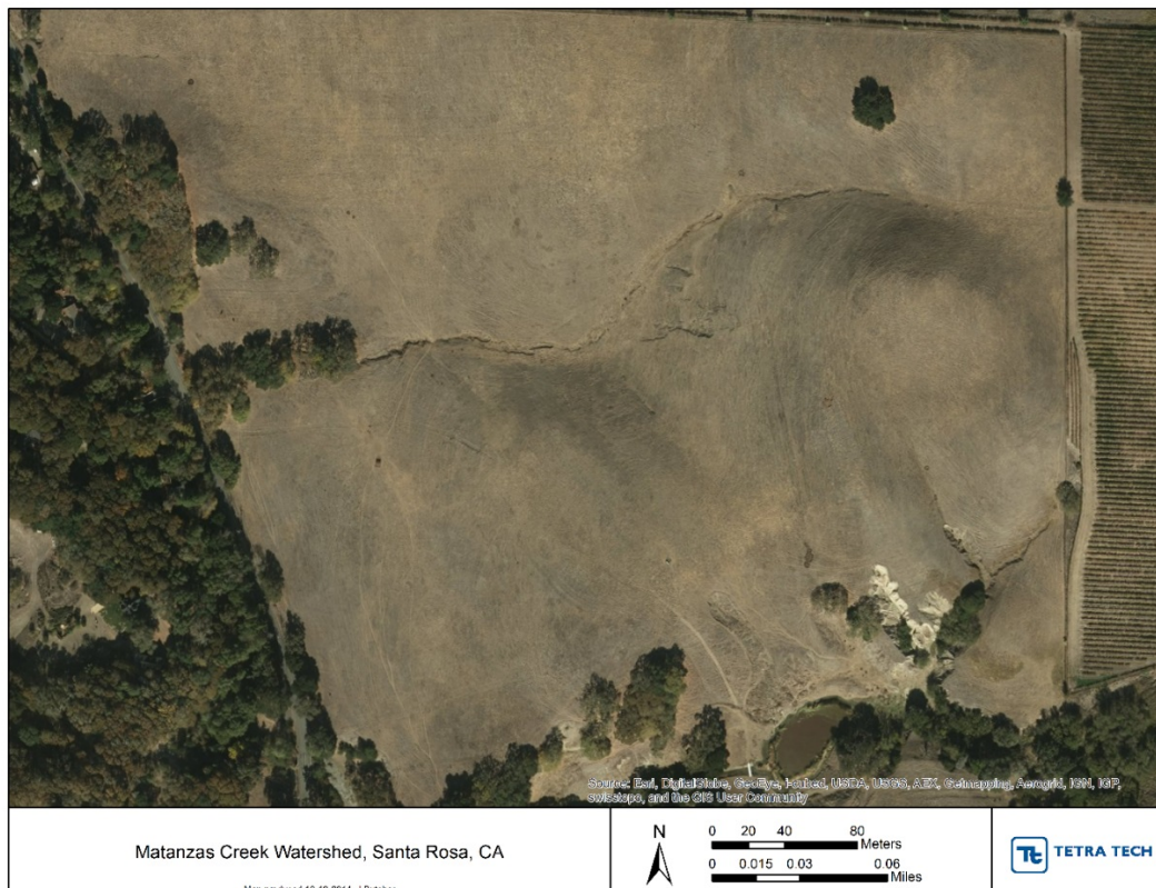
Figure 7-1. Example of Enlarging Gullies upstream of Matanzas Reservoir
