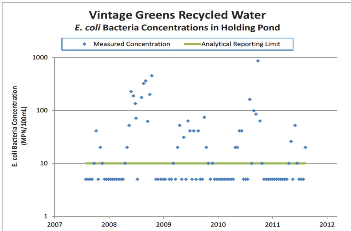
Figure 5.13: *E. coli* Bacteria Concentrations in a Recycled Water Holding Pond at Vintage Greens in Windsor
