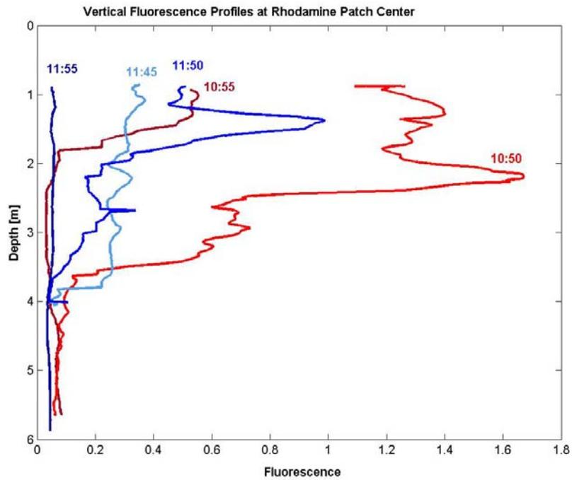
**Figure 50. Dispersion of rhodamine dye in Bodega Harbor, Fall 2003, rear channel (Porto Bodega).
