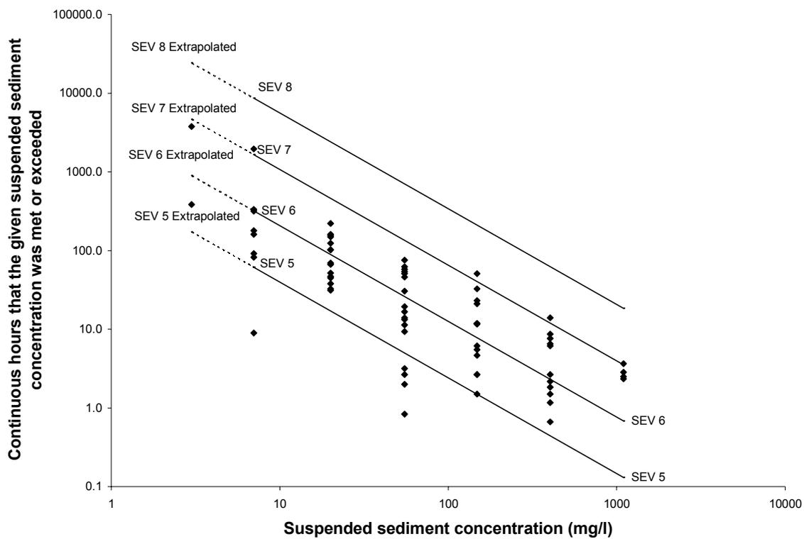
Figure 31. Continuous hours that a given suspended sediment concentration was met or exceeded at South Branch North Fork Elk River accompanied by Newcombe and Jensen model 1 severity of ill effects index (SEV) values for juvenile and adult salmonids.
