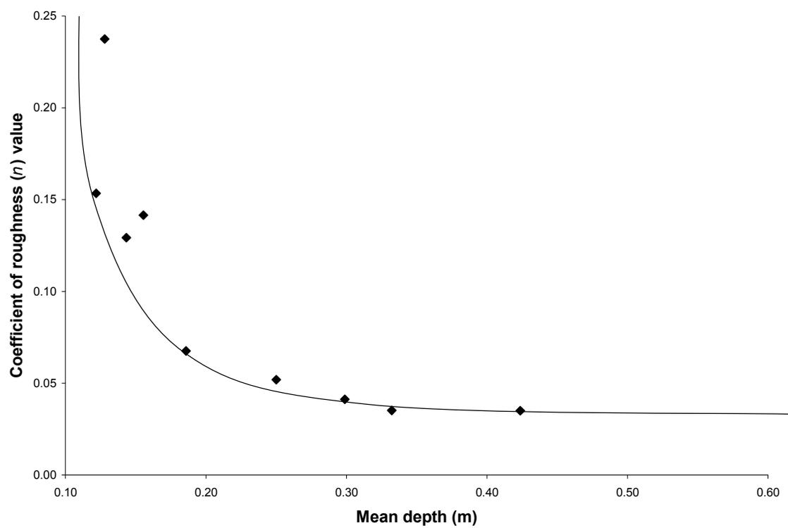
Figure 7. Computed coefficient of roughness ( $n$ ) values against mean depth for discharge measurements at Corrigan Creek.
