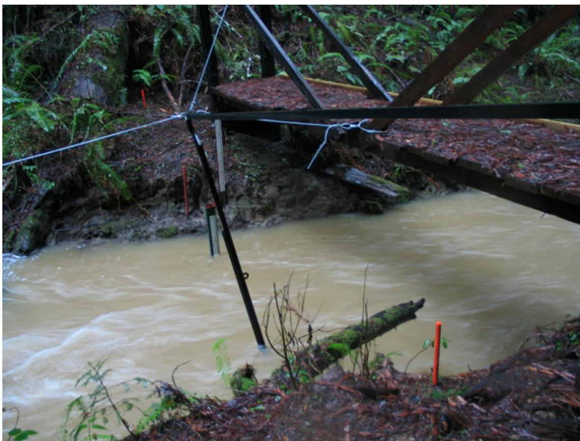
Figure 6. Bank mounted sampling boom articulating downstream during a high flow event on Corrigan Creek.
