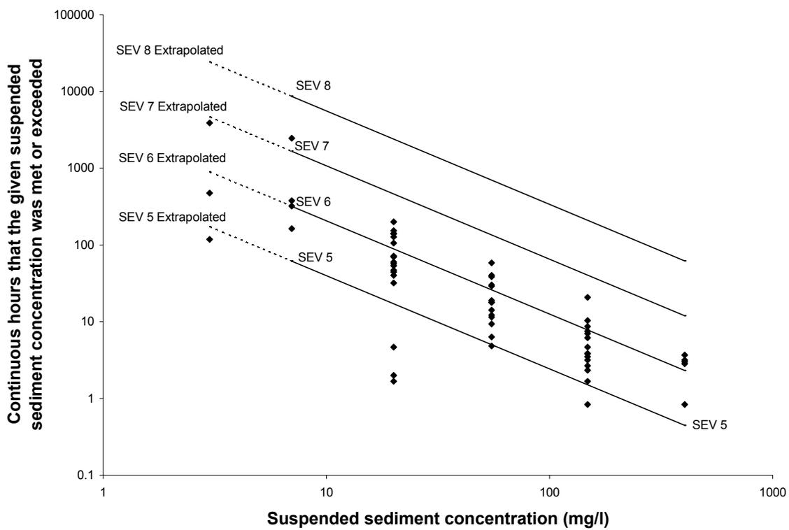
Figure 29. Continuous hours that a given suspended sediment concentration was met or exceeded at Corrigan Creek accompanied by Newcombe and Jensen model 1 severity of ill effects index (SEV) values for juvenile and adult salmonids.
