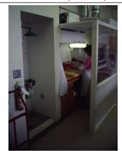
HEPA-filtered positive pressure clean room at the SCWA laboratory where the columns were prepared and eluted in a particle-free environment. The flexible plastic door is not visible in this photo.
