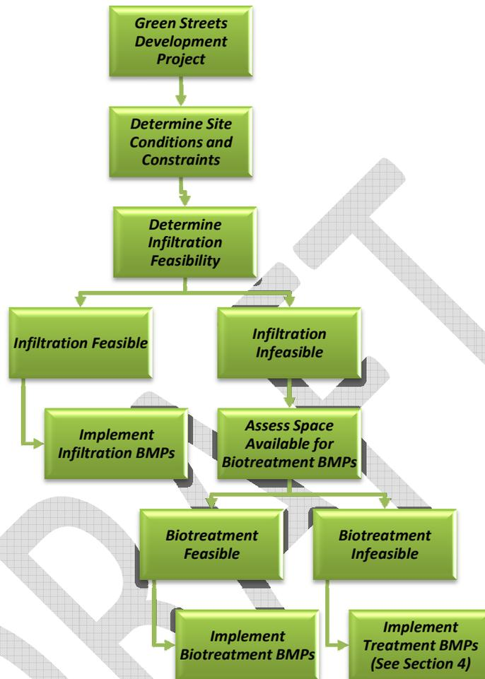
Figure 1: Flow Chart to Determine BMP Selection.
