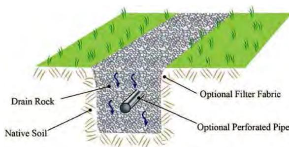
Figure 3: Infiltration Trench (*Model for Living Streets Design Manual, 2011*).
