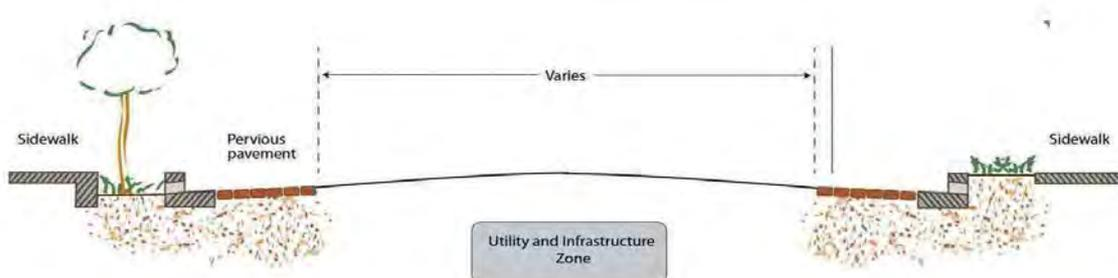
Figure 6: Possible pervious pavement design layout (*Model for Living Streets Design Manual, 2011*).
