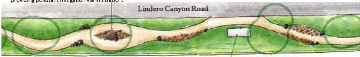
Figure 2: After Photo showing bio-swale eliminating runoff and providing pollutant mitigation via infiltration.
