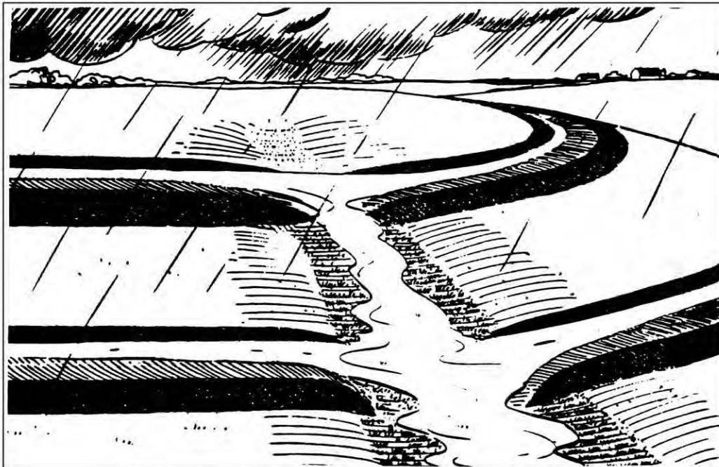
Figure 4c-5. Gradient terraces with waterway outlet (USDA-SCS, 1984).
