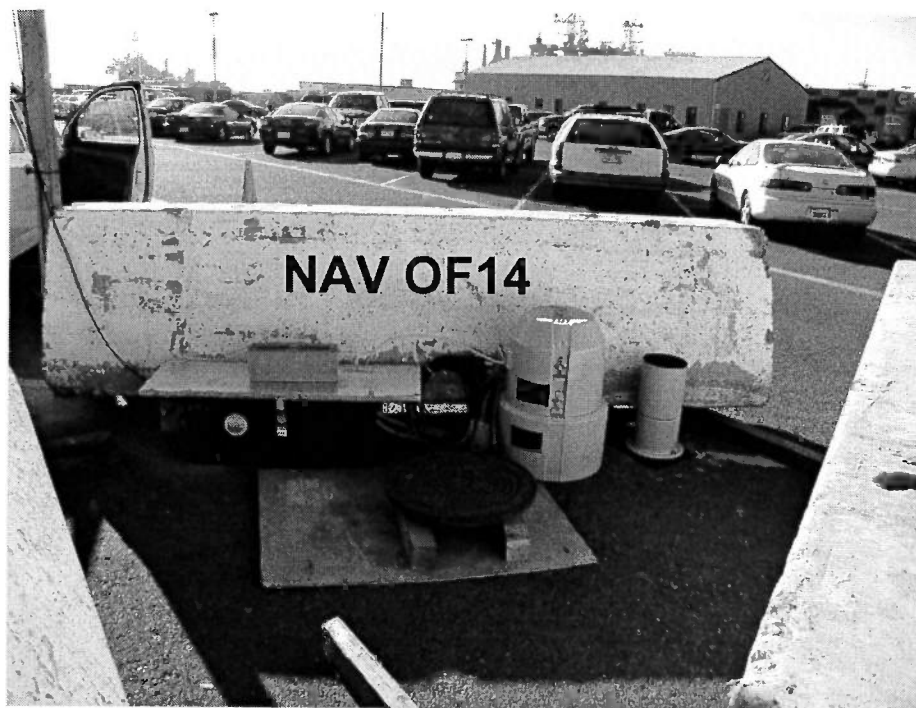
Figure 9. Naval Station San Diego storm water monitoring location for outfall 14. The site was located in a parking lot about 650 feet from the discharge point through the quay wall. The barriers were provided by the base to provide a secure monitoring area.
