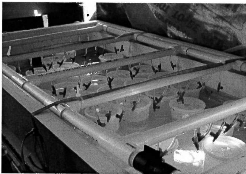
Figure 21. Flow-through bioassay setup aboard RV ECOS. Water was continuously dripped into each of the treatment beakers containing topsmelt, mysids, or mussel embryo larvae.
