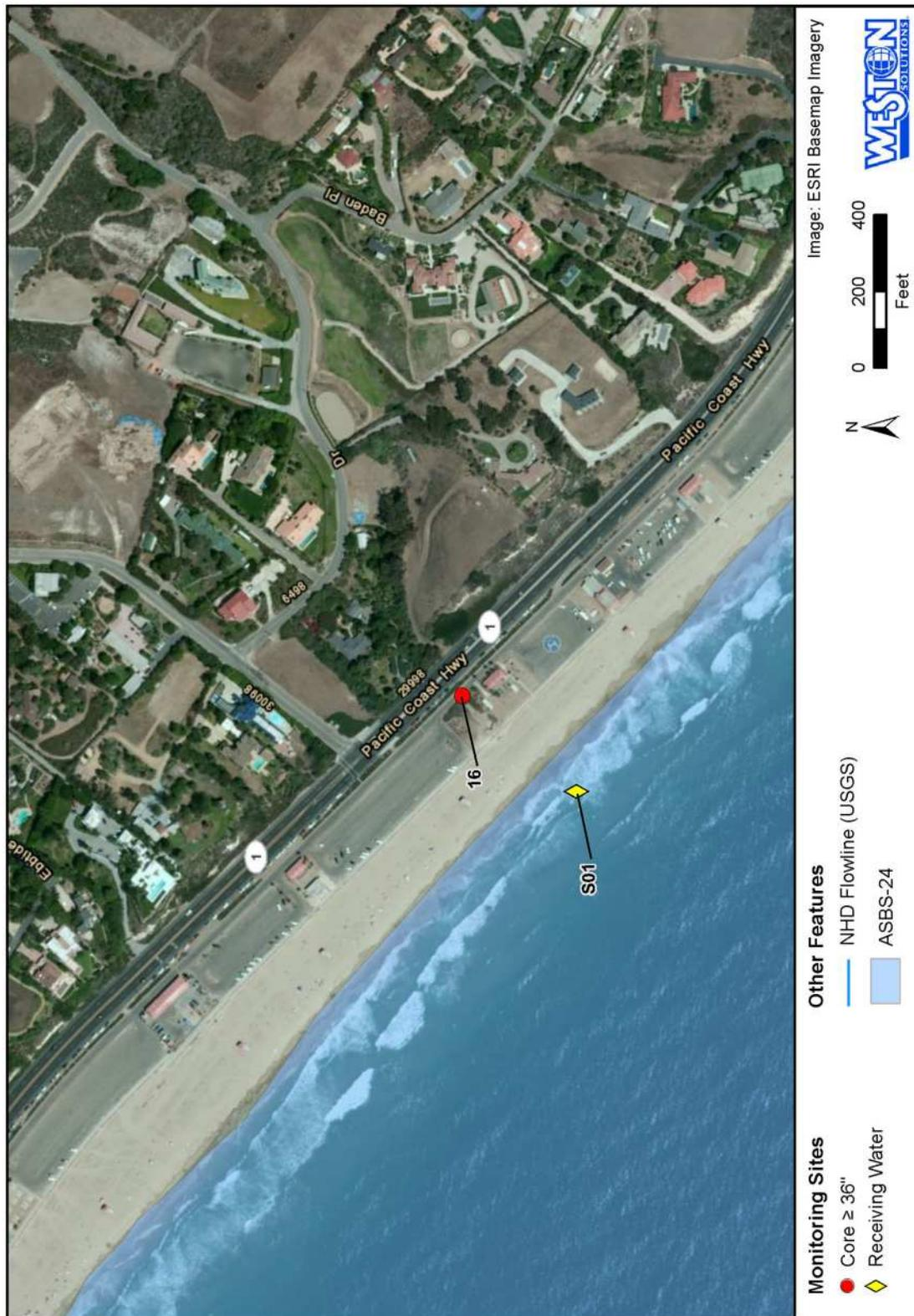
Figure 2-2. Core Discharge and Ocean Receiving Water Monitoring Locations along Zuma Beach
