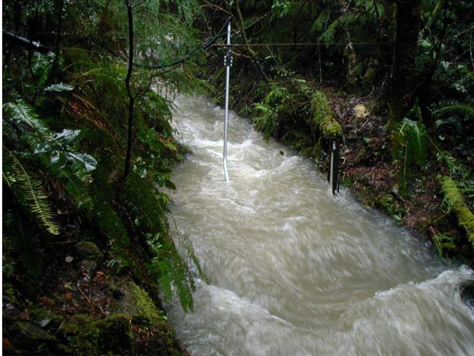
Photo 4. SF Wages above Center Gulch on 2/17/04 with a discharge of ~55 cfs. In this photo turbidity probe readings are being affected by turbulence. Boom has since been moved towards the right bank and out of the turbulence.
