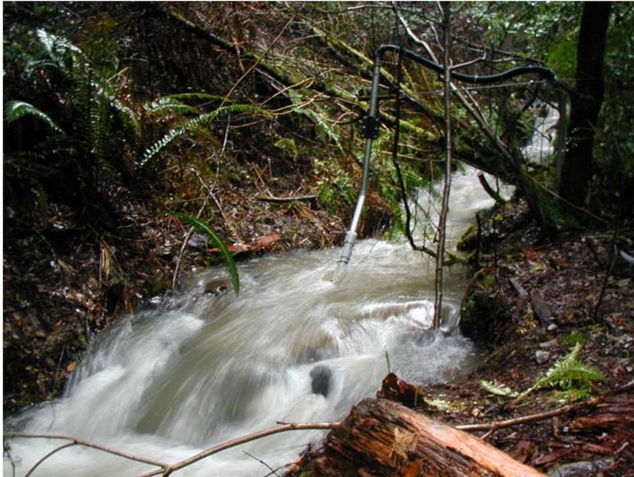
Photo 6. Center Gulch on 02/17/04 with a discharge of ~13 cfs. Photo taken after boulders were added to channel in order to backwater turbidity probe.
