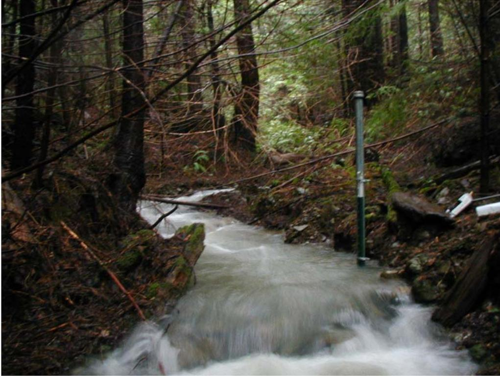
Photo 14. Grey Creek on 2/17/04 with a discharge of ~8 cfs. Note Crest Gage on left Bank. A rock weir was built to allow stage measurements.
