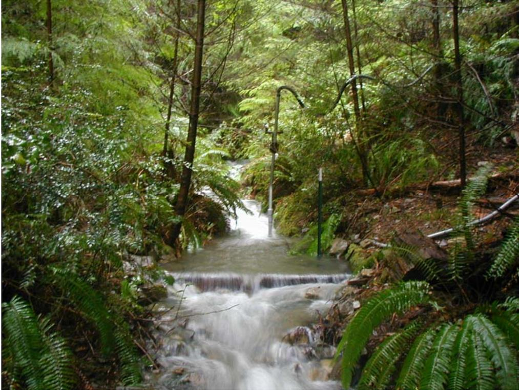
Photo 8. Wood above SF Wages on 2/17/04 with a discharge of ~5 cfs. In this photo turbidity probe readings are being affected by turbulence. Boom has since been moved towards the right bank and out of the turbulence.
