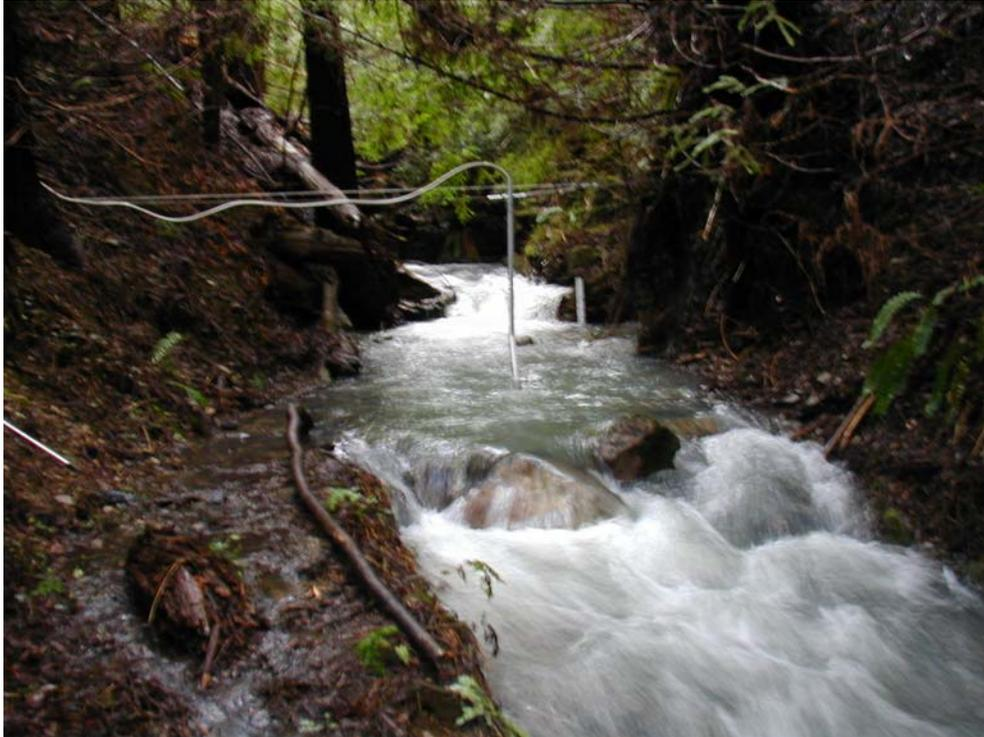
Photo 12. SF Wages above Rock Creek on 2/18/04 with a discharge of ~17 cfs. Note that large boulders placed in channel are working well at backwatering the turbidity probe.
