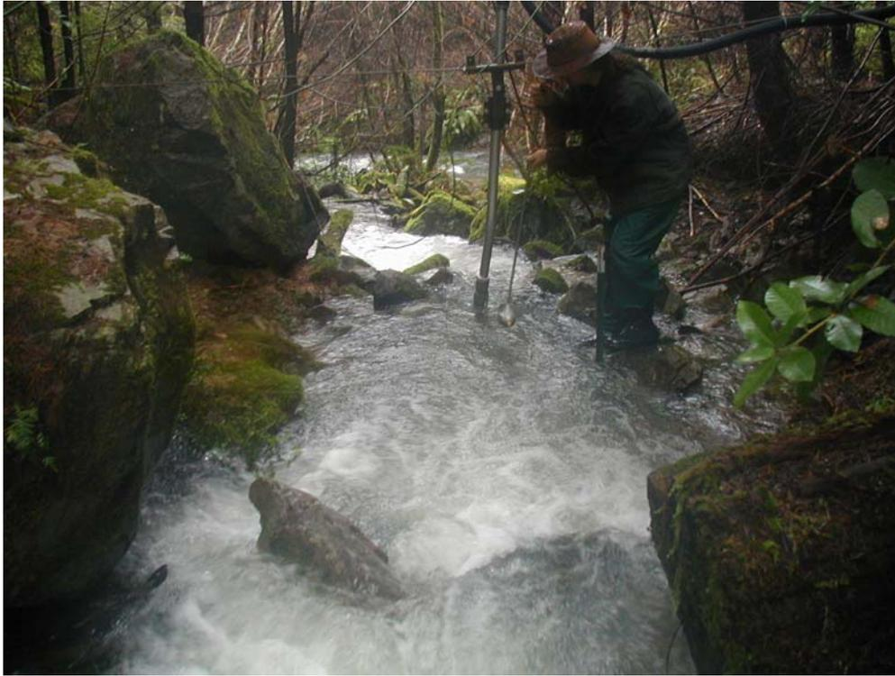
Photo 10. Rock Creek on 2/17/04 with a discharge of ~14 cfs. Hydrologist is performing DIS sediment sample with a DH-48.
