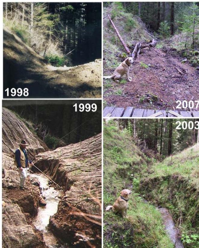
**Figure 3. Treated crossing CX-7 eroded severely and has yet to stabilize. In 2006, a debris flow deposit filled much of the void.**
