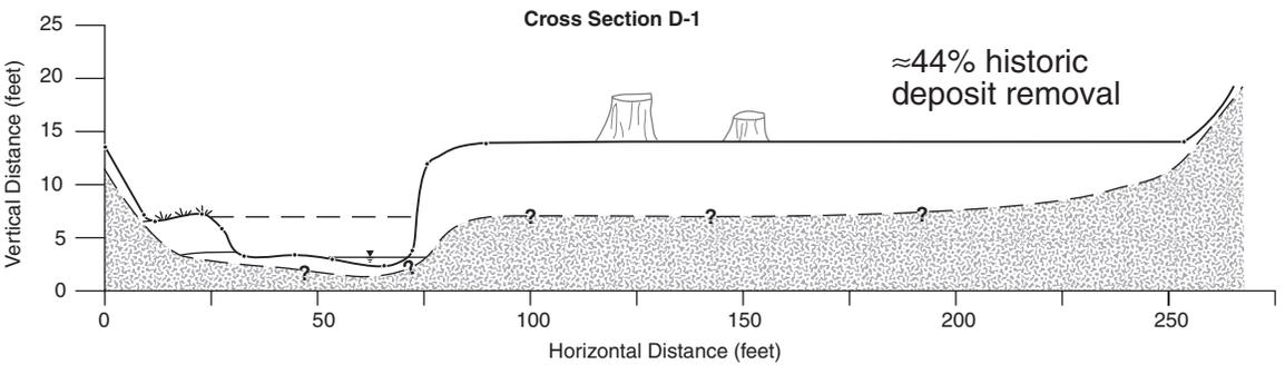
Figure 16. Surveyed cross sections B-1, C-1, and D-1. Dashed lines represent probable maximum thickness of historic aggradation used to estimate amount of material removed since time of terrace deposition.
