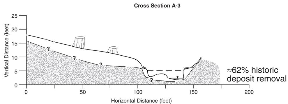
Figure 15. Surveyed cross sections A-1, A-2, and A-3. Dashed lines represent probable maximum thickness of historic aggradation used to estimate amount of material removed since time of terrace deposition.
