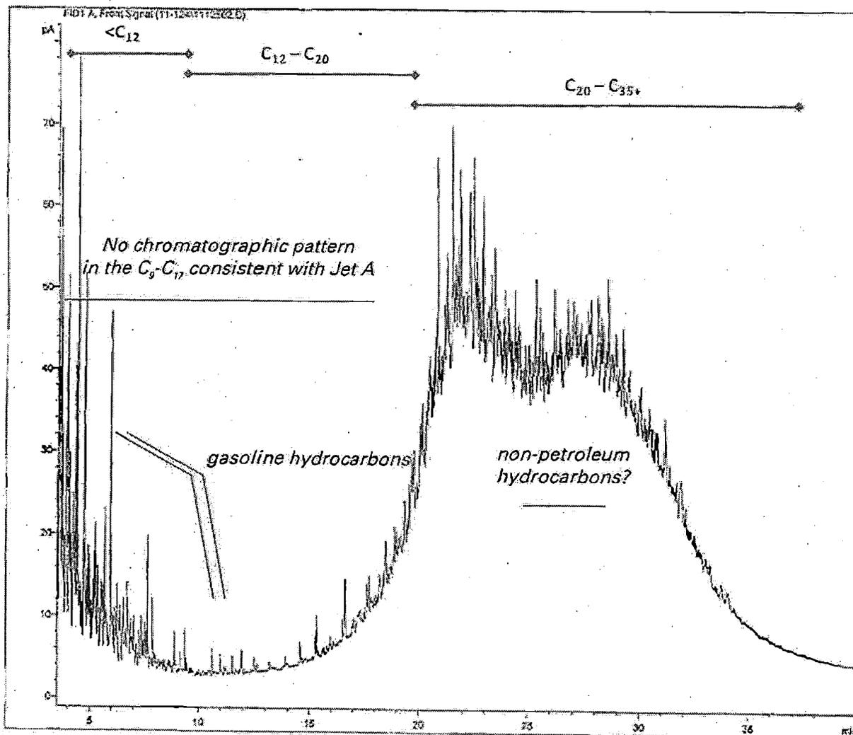
Figure 4. USCG Marine Safety Laboratory gas chromatogram of sample "CP-MW-2 (Source)". Preponderance of chromatographic signal is in the  $C_9-C_{12}$  range, and consistent in character with automotive gasoline. Small cluster of chromatographic peaks in the  $\sim C_{25}-C_{28}$  range are not readily recognized as a petroleum product; it is likely that these are hydrocarbons of some non-petroleum origin. There is no chromatographic evidence for the
