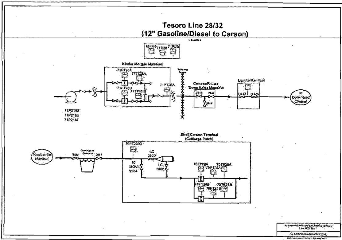
**FIGURE 2: SCHEMATIC DIAGRAM OF LINE 28/32 (GASOLINE/DIESEL PIPELINE)**
