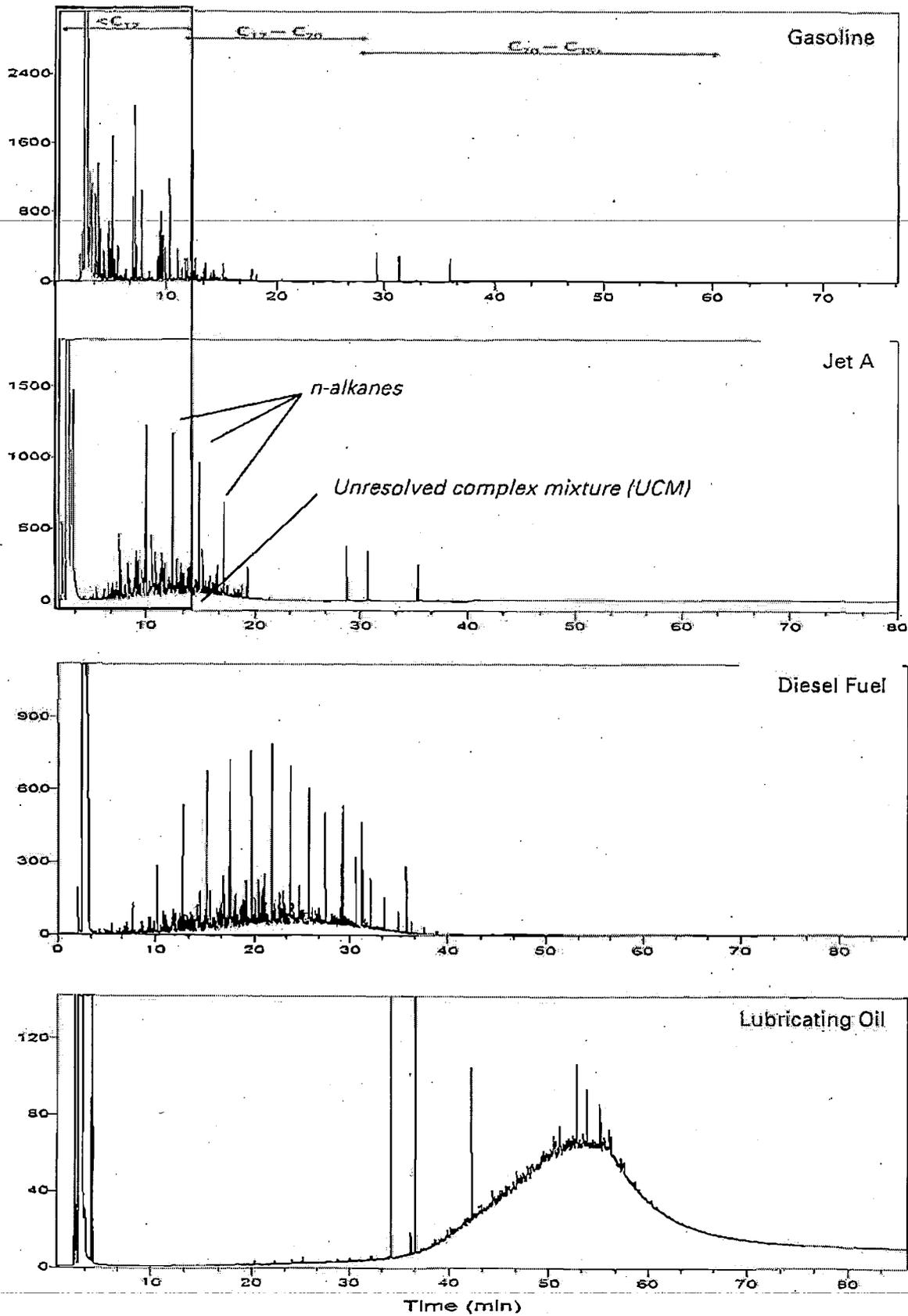
Figure 1. Comparative gas chromatograms and compositional carbon ranges for petroleum reference products. Note: shaded box shows  $C_9-C_{12}$  carbon range compositional "overlap" between gasoline and Jet A. Carbon ranges depicted.
