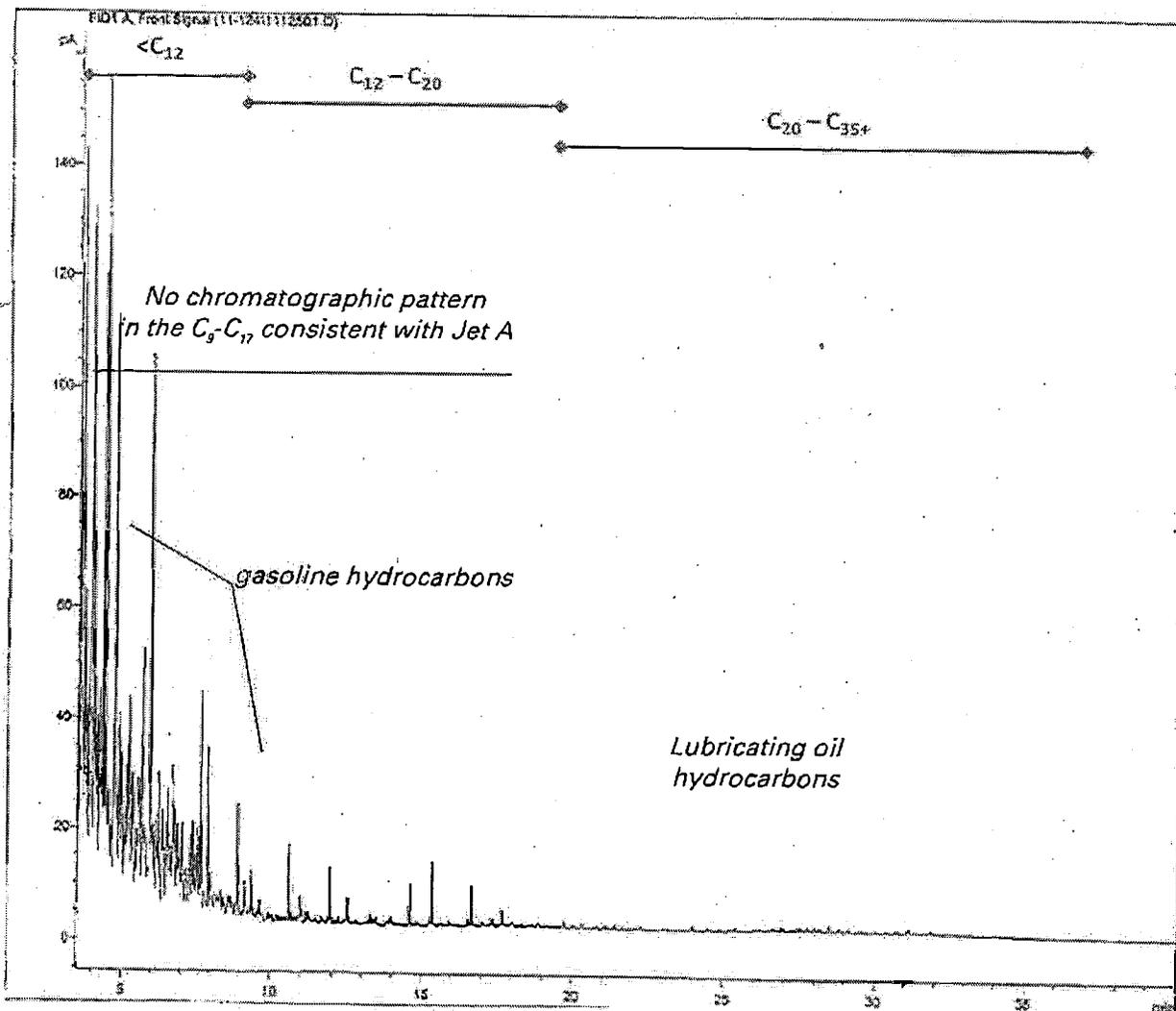
Figure 3. USCG Marine Safety Laboratory gas chromatogram of sample "CAH-MW-1 (Source)". Preponderance of chromatographic signal is in the  $C_{20}-C_{35+}$  range (consistent in character with complex mixture of lubricating oil), and  $C_9-C_{12}$  hydrocarbons consistent with automotive gasoline. There is no chromatographic evidence for the presence of Jet A.
