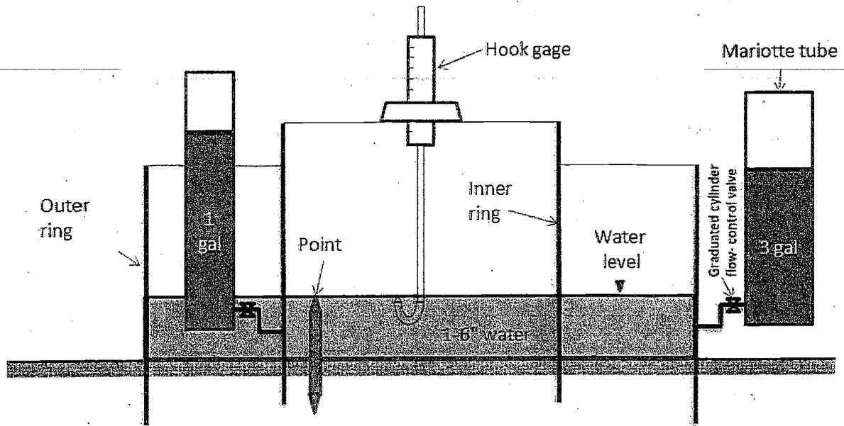
Figure VII.10. Double Ring Infiltrometer Set-up with Mariotte Tubes
