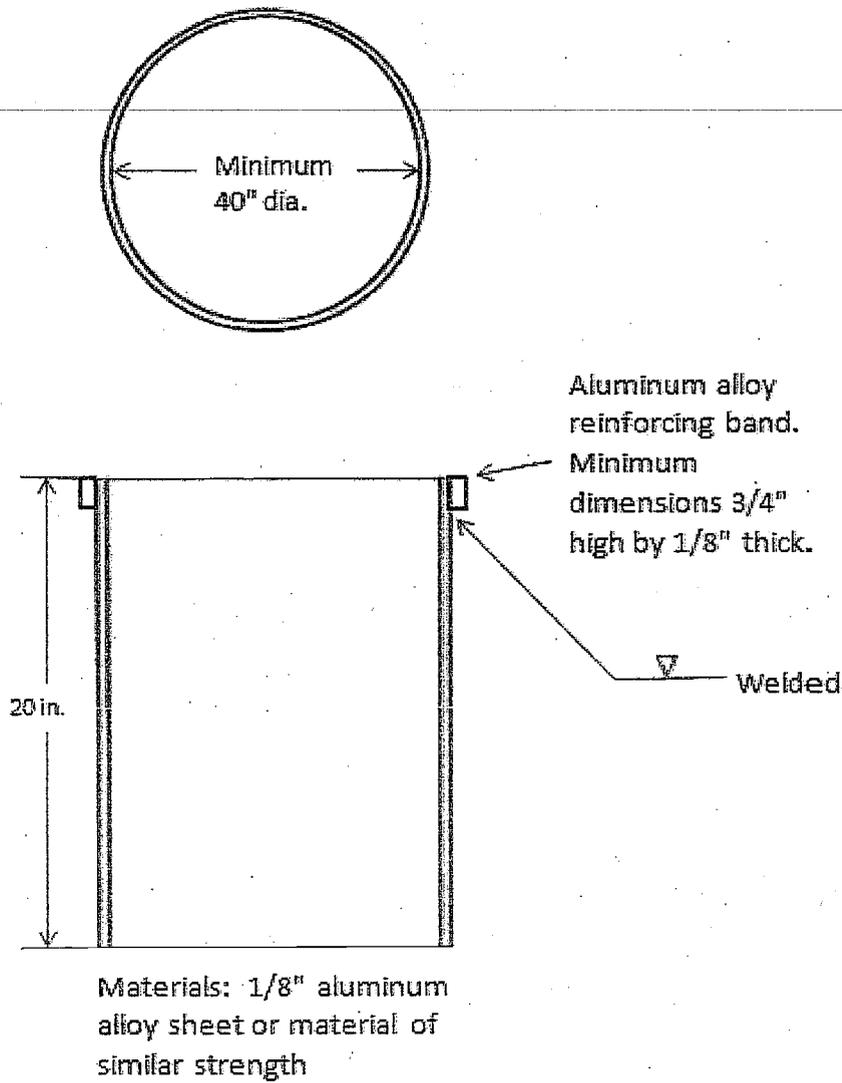
Figure VII.3. Single Ring Infiltrometer Setup with Mariotte Tube
