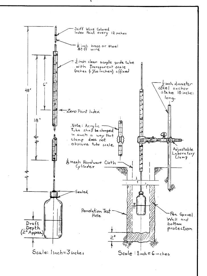
FIGURE B1. FLOAT GAGE AND PERCOLATION TEST ASSEMBLY
