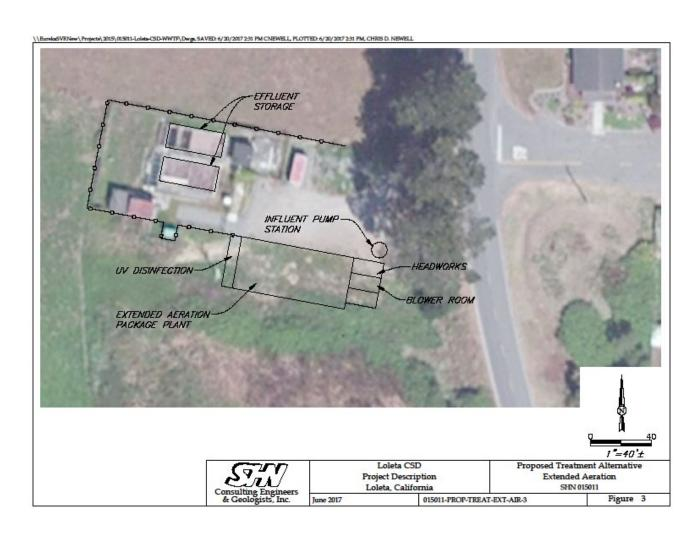
Figure B-3. Proposed Wastewater Treatment Facility Map
