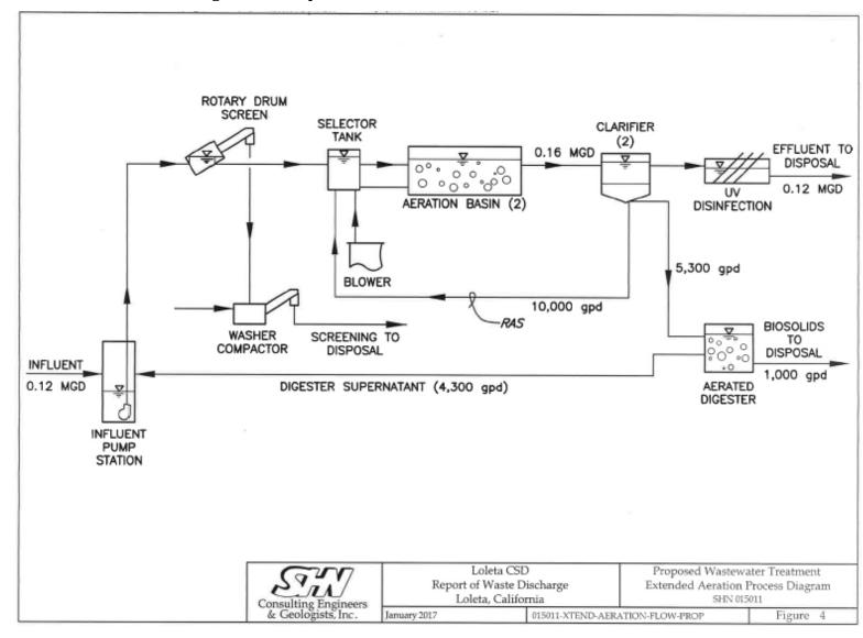
Figure C-2. Proposed Wastewater Treatment Flow Schematic
