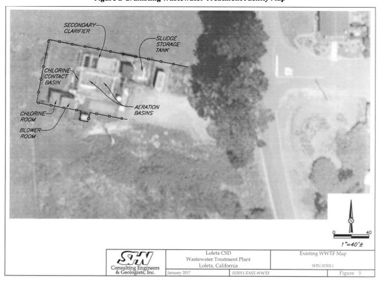
Figure B-2. Existing Wastewater Treatment Facility Map
