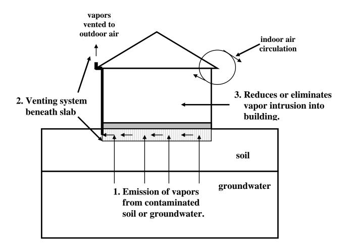
Figure 4. Typical vapor mitigation system.
