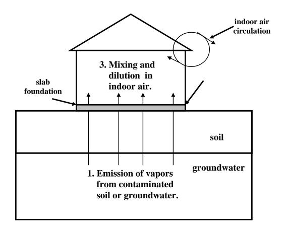
Figure 3. Model of vapor intrusion into buildings.
